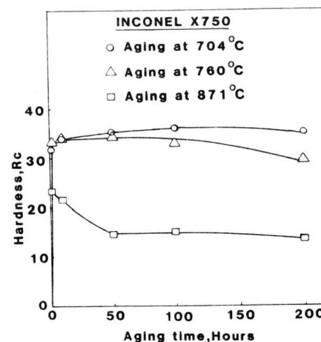
Fig. 1. Hardness versus aging time.
