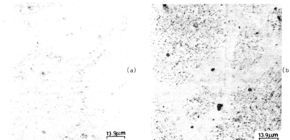
Fig. 2. Inconel X-750 solution treated, water quenched and aged at (a) 871°C, 2 hrs. and (b) 871°C, 200 hrs.
