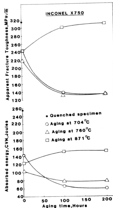
Fig. 4. Effect of aging time on impact properties of age treated Inconel X-750.
