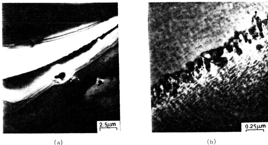
Fig. 3. Typical TEM microstructures corresponding to aging at 704°C for (a) 2 hrs. and (b) 100 hrs. aging times.
