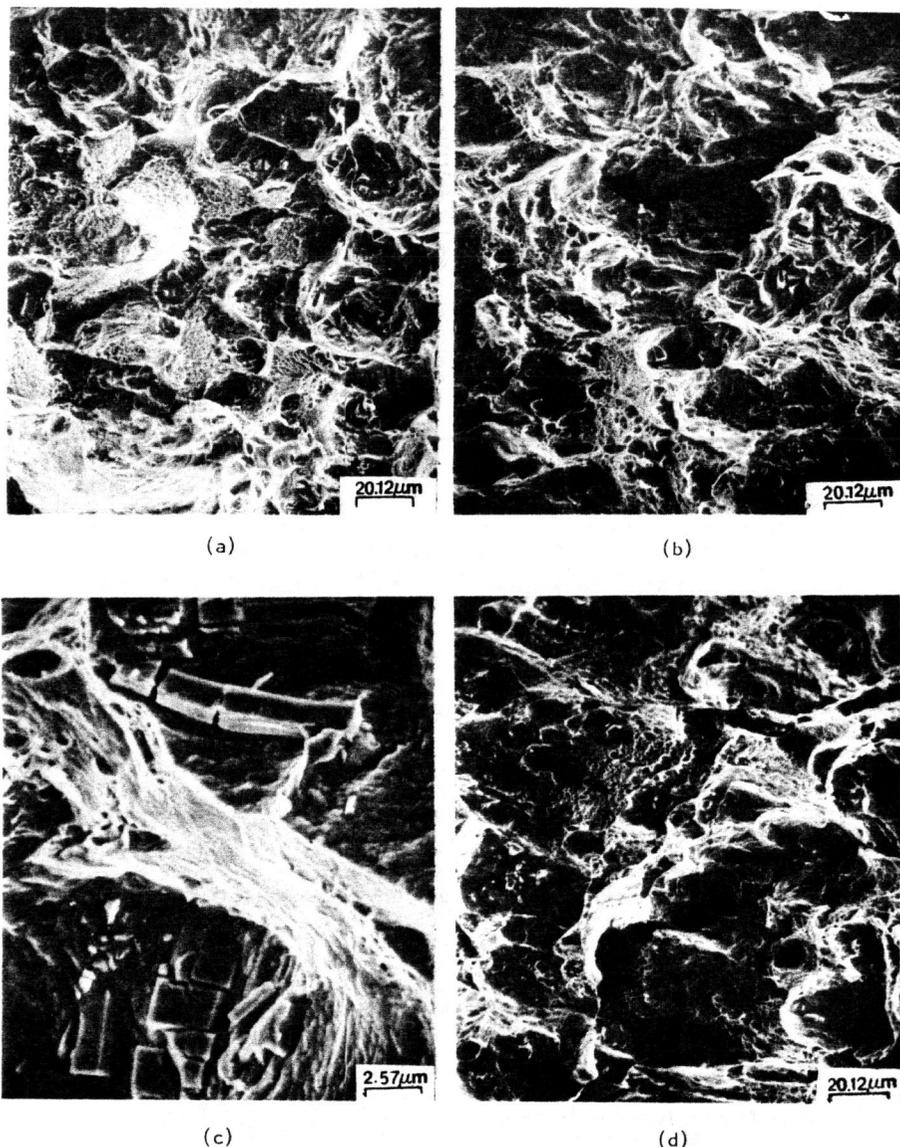
Fig. 7. SEM fractographs of impact specimens aged at (a) 871°C for 2 hrs., (b,c) 871°C for 100 hrs. at different magnifications, and (d) 871°C for 200 hrs.
