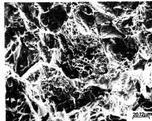
Fig. 6. SEM fractograph of impact specimen aged at 760°C for 2 hrs.
