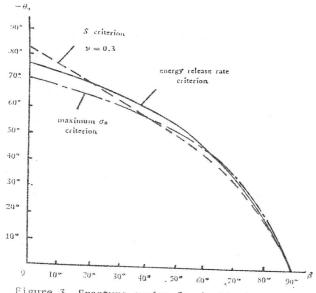
Figure 3 Fracture angles for inclined crack under uniaxial tension
