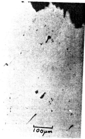
Figure 3 Longitudinal section of alloy BD6 after tensile fracture at 20°C (Optical micrograph unetched)
