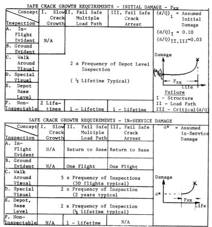
Figure 1 - Summary of Crack Growth Requirements
