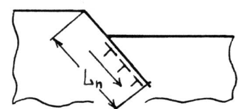
Fig1. Scheme of generation of effective dislocations near the surface
