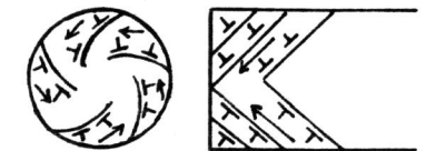
Fig3. Generation of effective dislocations during cross-rolling in cross (a) and not axial (b) sections
