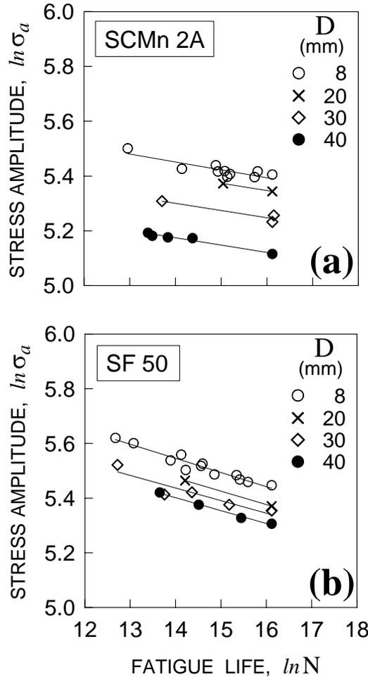
Figure 5. S-N curves related to two steels tested by Hatanaka et al.[14], for different values of specimen diameter  $D$ . Fatigue strength  $\sigma_a$  is expressed in MPa.
