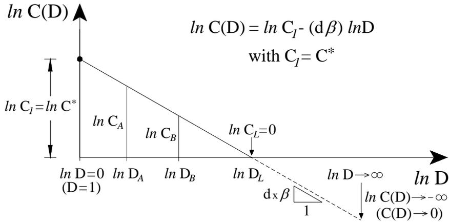
Figure 3. S-N curve parameter  $C(D)$  against structure size  $D$ .
