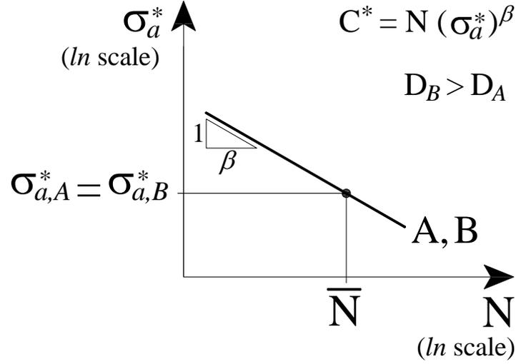
Figure 2. Fractal (or renormalized) S-N curve in a bilogarithmic diagram.
