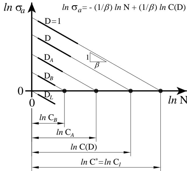
Figure 4. Finite-life fatigue strength  $\sigma_a$  against number  $N$  of loading cycles.
