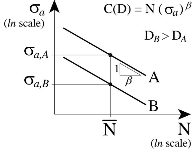
Figure 1. S-N curves in a bilogarithmic diagram.
