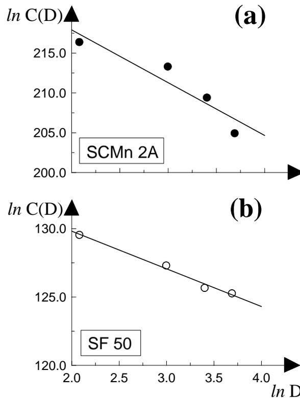
Figure 6. Experimental S-N curve parameter  $C(D)$  against structure size  $D$  for two steels tested by Hatanaka et al. [14].
