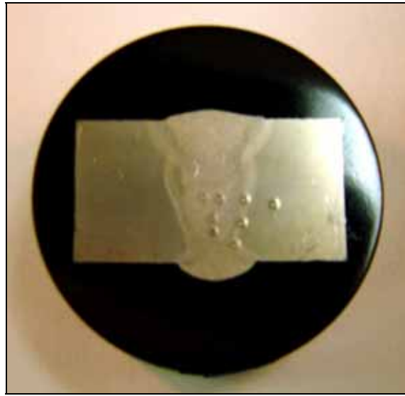
Fig. 5 ABI tests on base metal, girth weld, and HAZ areas of high strength pipeline steel.
