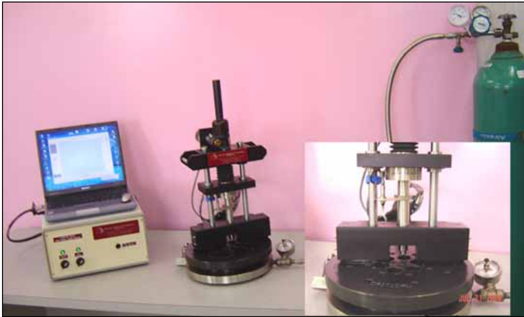
Fig. 6 Test set-up: SSM system, hydrogen chamber, and hydrogen cylinder.
