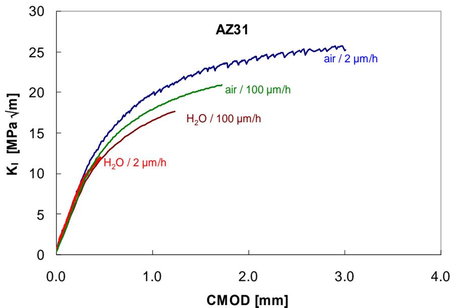
Fig. 3: Curves of the stress intensity factor,  $K_I$ , vs. crack mouth opening displacement, CMOD, measured in tests on pre-cracked C(T) specimens of the Mg alloy AZ31 at two extension rates in distilled water and in laboratory air and plotted up to the onset of cracking observed in each test.
