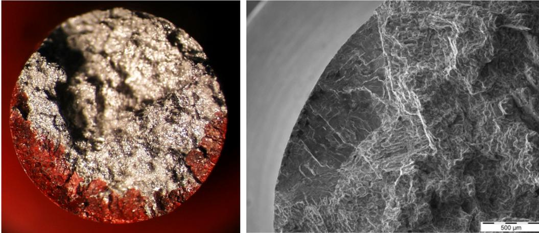
Fig. 2: Fracture surfaces of an AZ91 tensile specimens tested under constant load in distilled water, showing areas of hydrogen induced cracking; left: optical microscope, right: scanning microscope.
