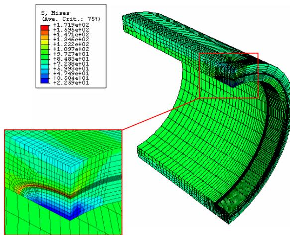
Fig.4. FE-Model of tube with a half-elliptical crack
