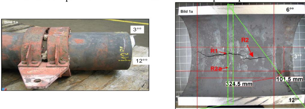
Fig. 2: Damage area of the bent tube, internal side of the pipe [9]
