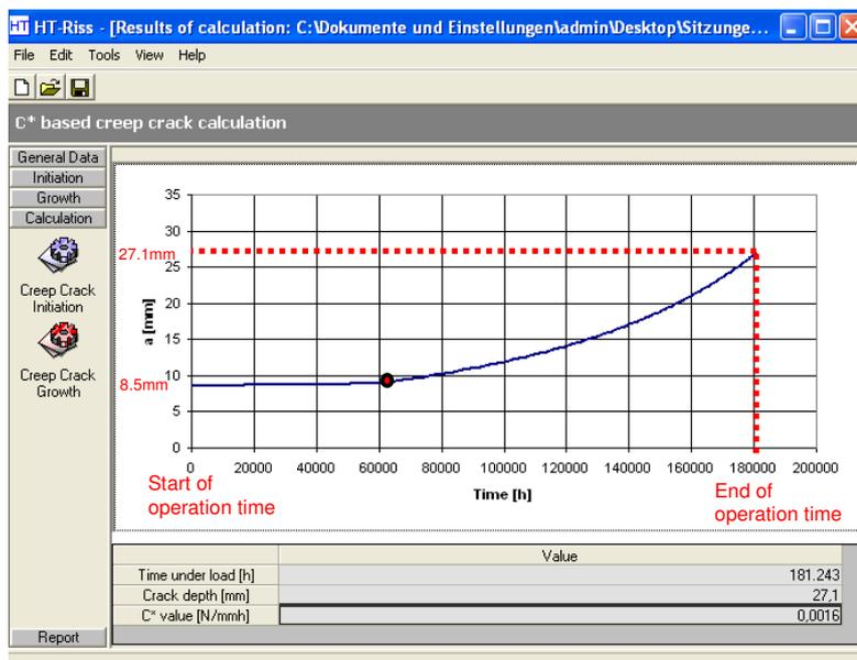
Fig. 5: Calculation result for the half-elliptic crack R1
