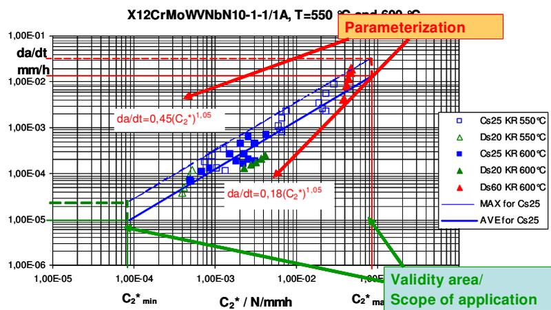
Fig. 1: Material data for X12CrMoWVNbN10-1-1 / 550°C and 600°C, here: creep crack growth depending on the  $C^*$ -parameter.
