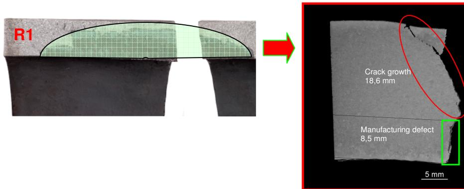
Fig. 3: Crack configuration at the metallographic specimen through the pipe wall, crack R1
