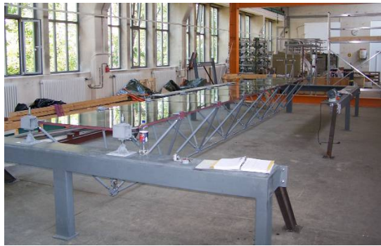
Figure 3: Completed 10 m roof mock-up.
