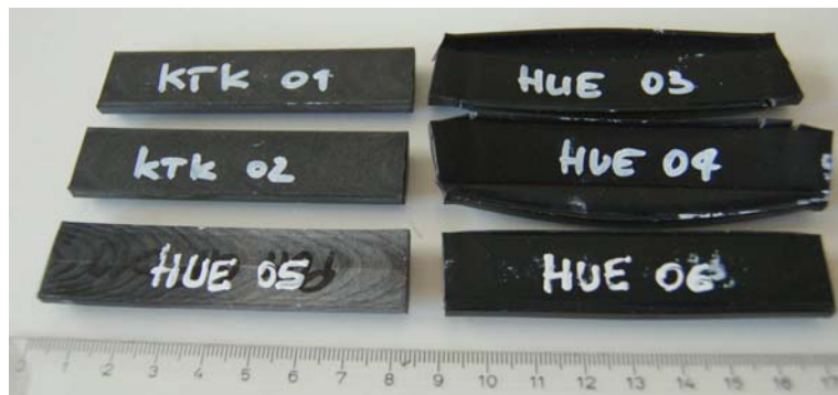
Figure 11: POM-C GF25 specimens (80 mm x 16 mm) of different fabricators.
