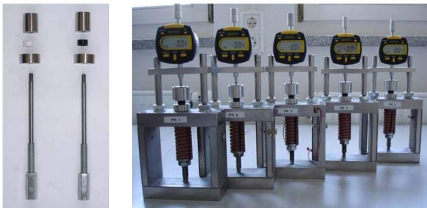
Figures 13a and 13b: Specimens and testing facility for creeping tests.
