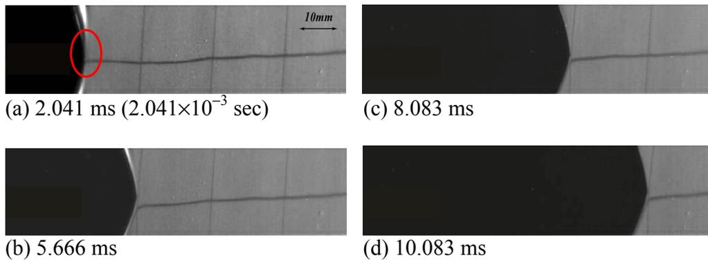
Fig.3. Typical hyperelastic dynamic rupture propagation recorded experimentally utilizing a high-speed digital video camera (under uniaxial tension; extension ratio:  $\lambda_y = 3.0$ ; final rupture speed: 11 m/s). Elapsed time after rupture initiation is indicated in milliseconds. The initial thickness of the rubber sheet is 1 mm and the lines are drawn for the observational purpose.
