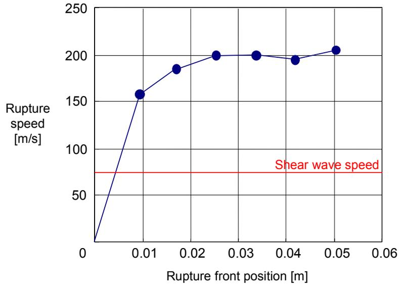
Fig.6. History of rupture speed: Supershear case. Similar to the subsonic case, the rupture speed increases immediately after initiation and approaches a final constant value exceeding the shear wave speed.
