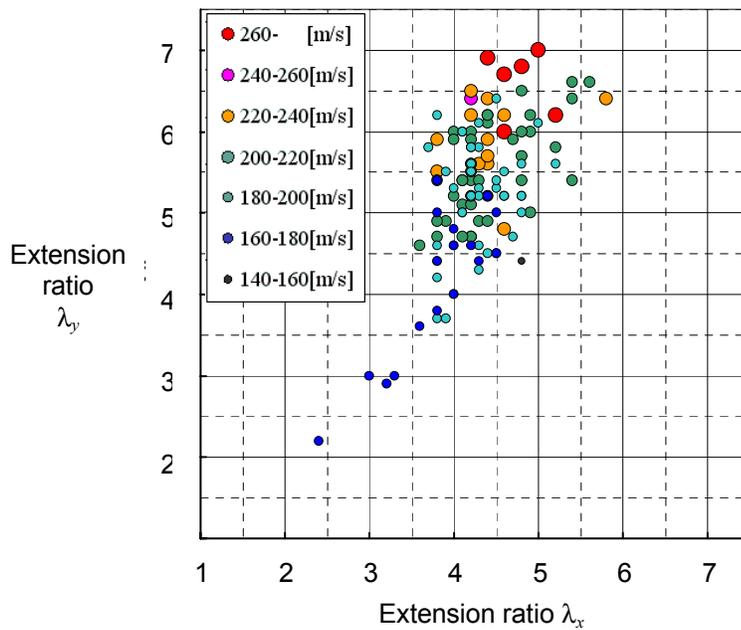
Fig.7. The (final constant) speed of stably propagating rupture under various extension ratios. Similar to the linear elastic case, higher  $T$ -stress ( $\lambda_x$ ) generally gives more stability of rupture propagation and thus renders larger rupture speed, but the extension ratio  $\lambda_y$ , measured perpendicular to the rupture direction, has also strong influence on the propagation speed.
