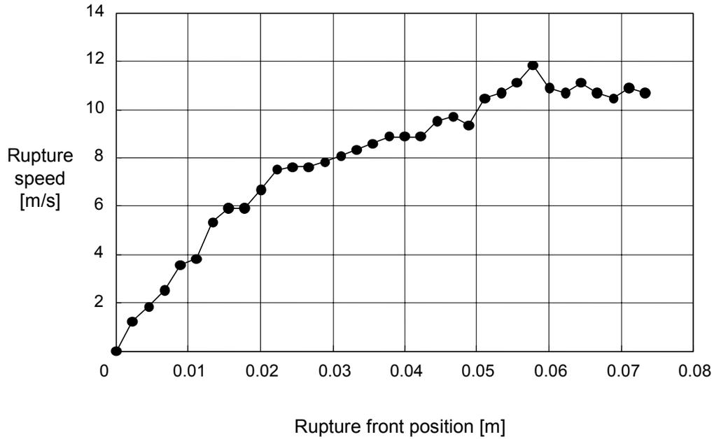
Fig.4. History of the speed of the rupture front: Subsonic case. Upon initiation, the rupture speed increases fast and approaches a constant value.
