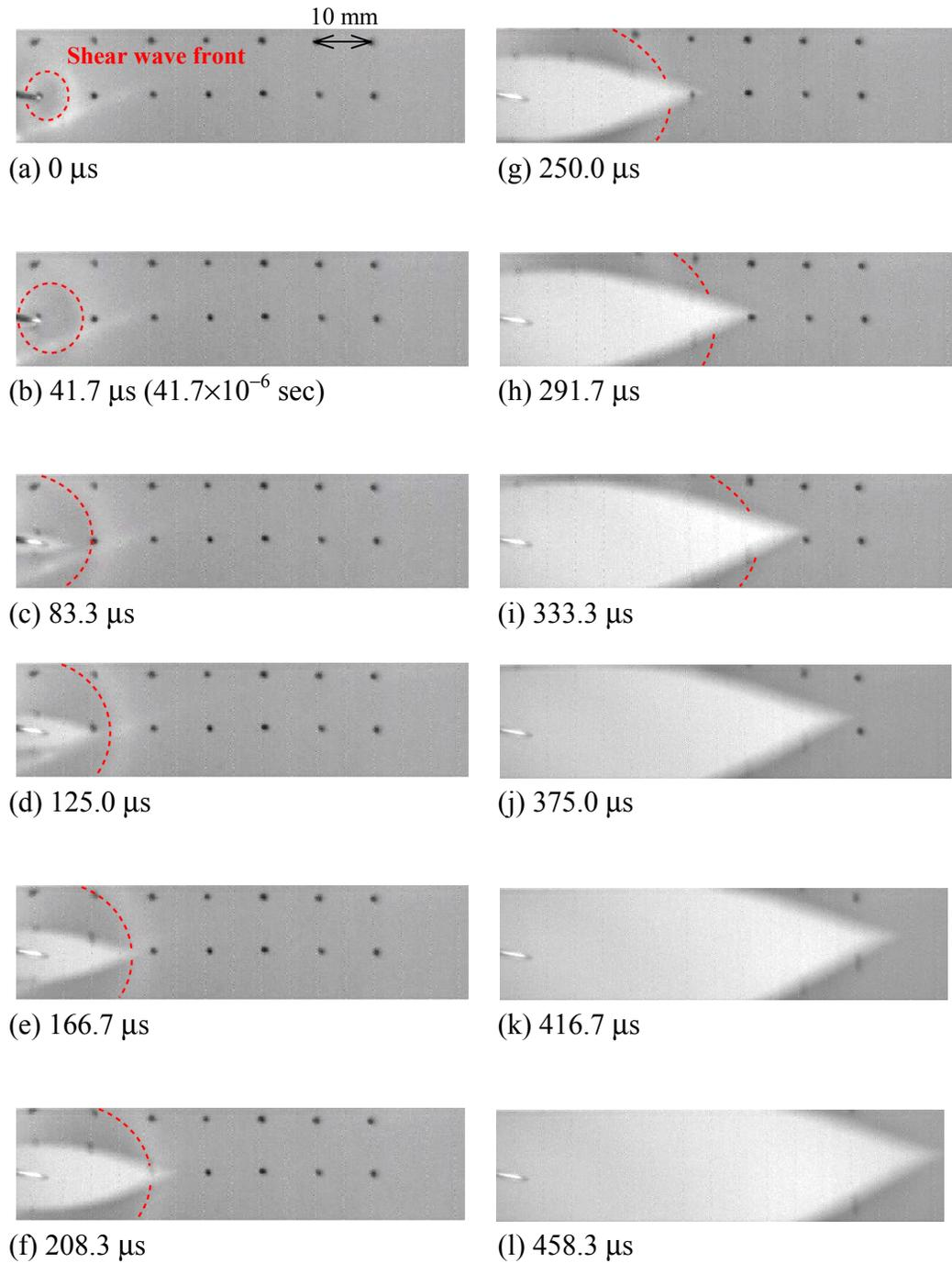
Fig.5. The dynamic rupture process recorded by the high-speed digital video camera system. These photographs show that the rupture speed becomes larger than the (shear) wave speed (extension ratios:  $\lambda_x = 4.0$ ,  $\lambda_y = 4.0$ ; final rupture speed: 181 m/s; wave speed: 75 m/s; initial thickness of the rubber 2.2 mm). The red broken lines correspond to the wave fronts. Elapsed time after rupture initiation is given in microseconds.
