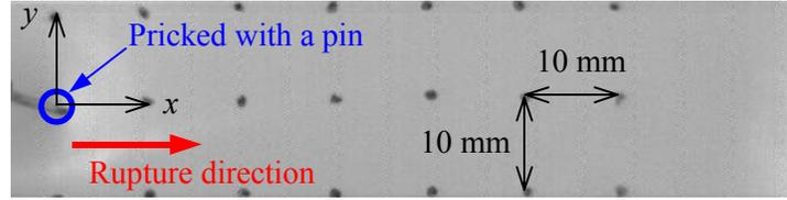
Fig.1. The definition of  $x$ - and  $y$ -axes. The rupture is initiated by prick of a pin and propagated in the  $x$ - direction of the hyperelastic rubber sheet.
