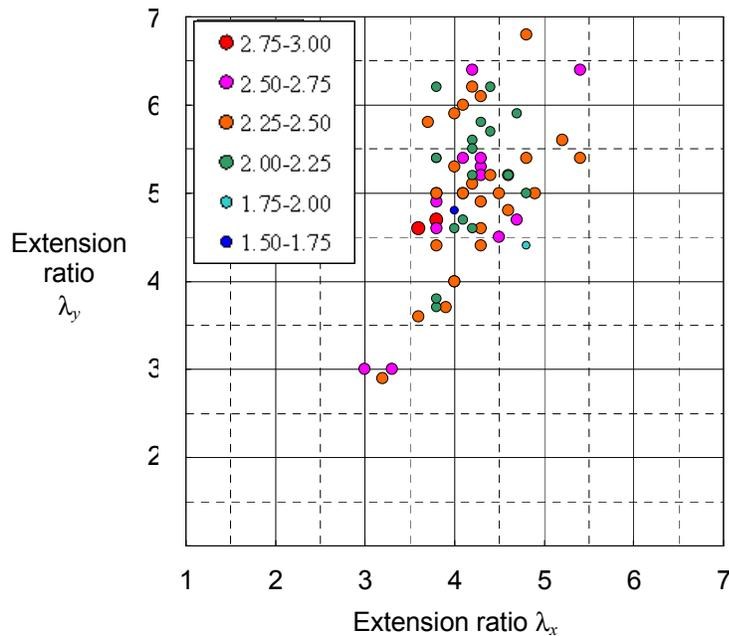
Fig.9. The Mach numbers (the ratio of rupture speed to shear wave speed) obtained experimentally in a monolithic medium, under different extension ratios. In hyperelastic media, Mach numbers over 2 can be commonly observed.
