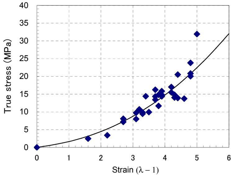
Fig.2. The true stress-strain relation of the rubber under biaxial loading ( $\lambda_x = \lambda_y = \lambda$ ). The experimentally obtained result is indicated by dots. We notice rather strong strain-hardening effect. The solid curve is drawn for the theoretical stress-strain relation in the Generalized Neo-Hookean (GNH) model, with the shear modulus  $\mu = 0.3$  MPa, "yielding" parameter  $b = 1$  and the "hardening" parameter  $n = 1.15$ .
