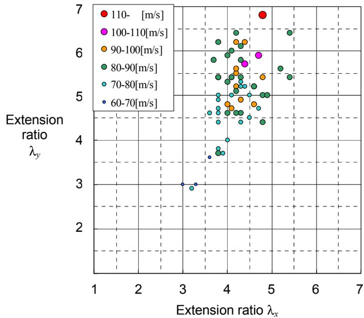
Fig.8. The experimentally observed shear wave speeds under different combinations of extension ratios. As can be expected from the nonlinear stress-strain relation shown in Fig.2, higher extension ratios generally give larger wave speed.
