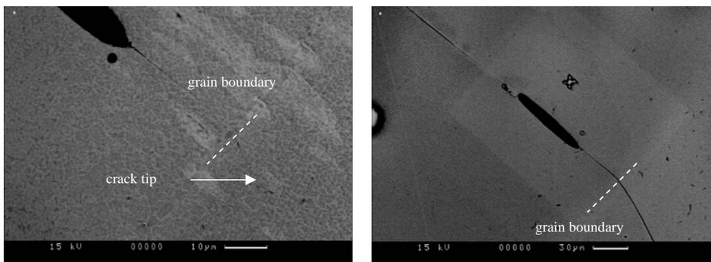
**Fig.6a)** The notch has a distance of 30  $\mu\text{m}$  to the grain boundary.
