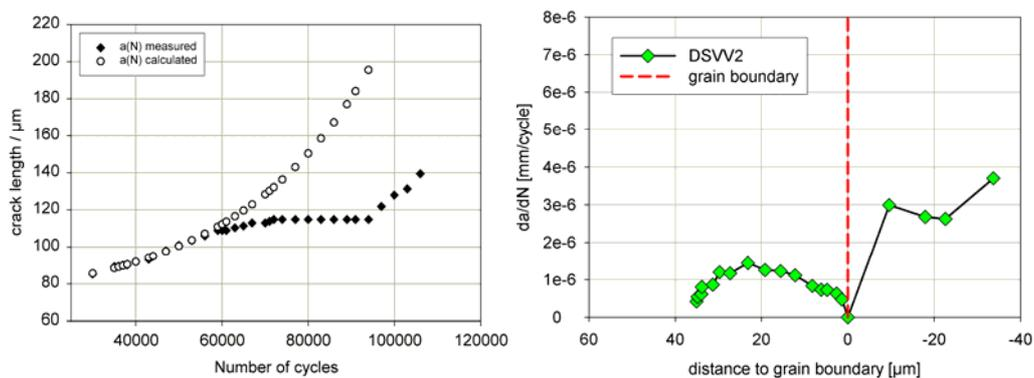
**Fig.3 a)** Crack length as function of the number of cycles as measured and as calculated for a specimen without grain boundary.
