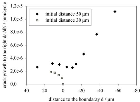
**Fig.8:** Crack advance for the part of the crack facing the boundary related to the distance
