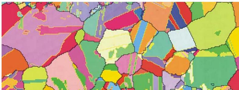
**Fig.1:** EBSD-grain orientation map of a polycrystalline nickel specimen. Twin boundaries are marked in yellow (not in print version available).
