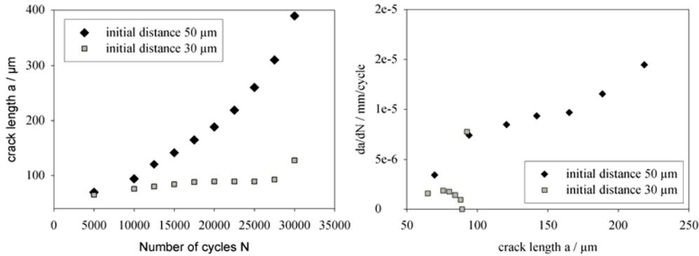
**Fig.7 a)** Crack length as a function of cycles for both cracks.
