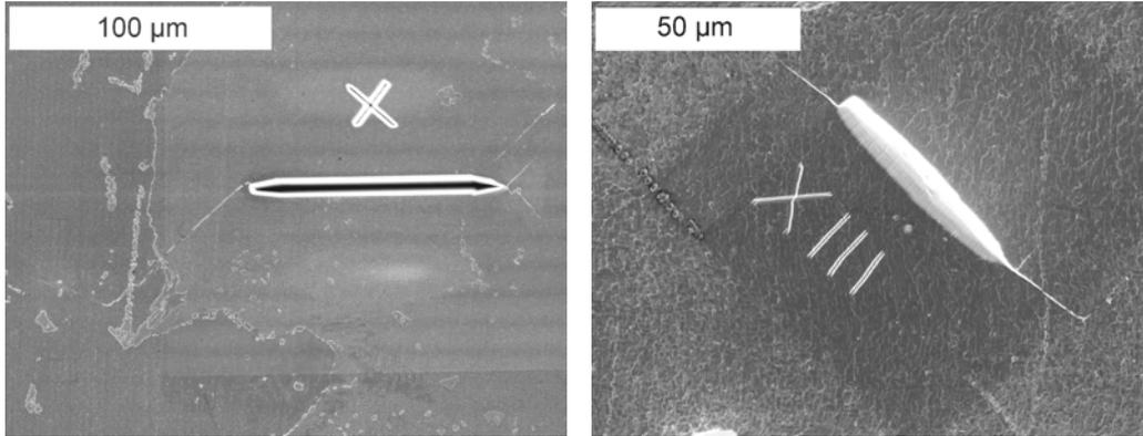
**Fig.2a)** FIB notch in front of a grain boundary with a crack emitted from the notch tip cutting the grain boundary.
