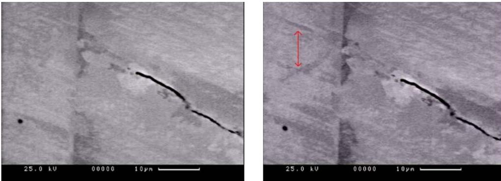
**Fig.4:**ECCI images of a crack tip in front of a grain boundary (going from the top to the bottom of the images).
