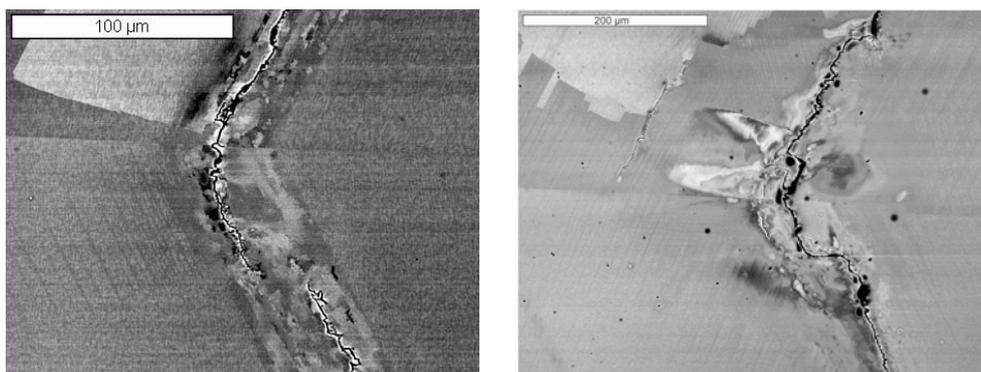
**Fig.5:** The plastic zone around two different cracks:
