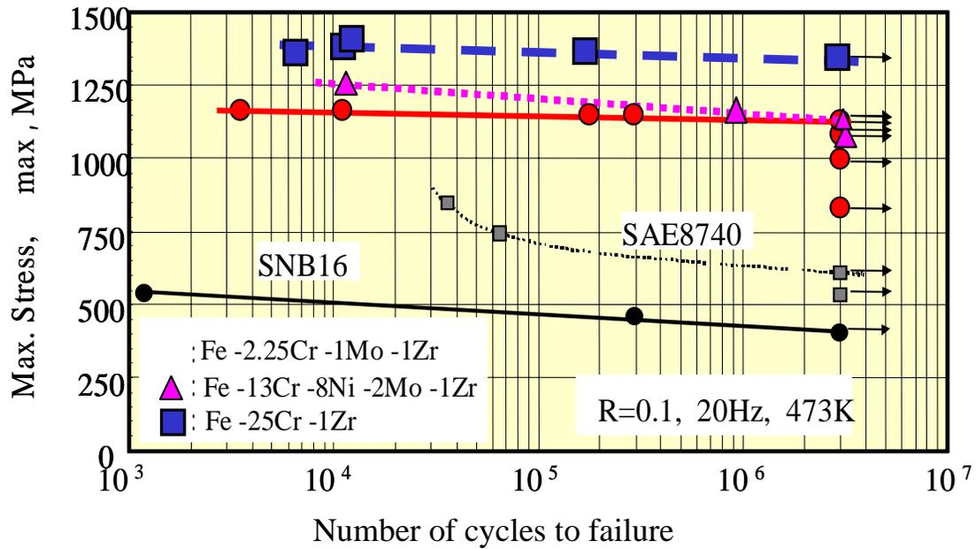
Fig.4 S-N diagrams of ultrafine grained ferritic stainless steels.
