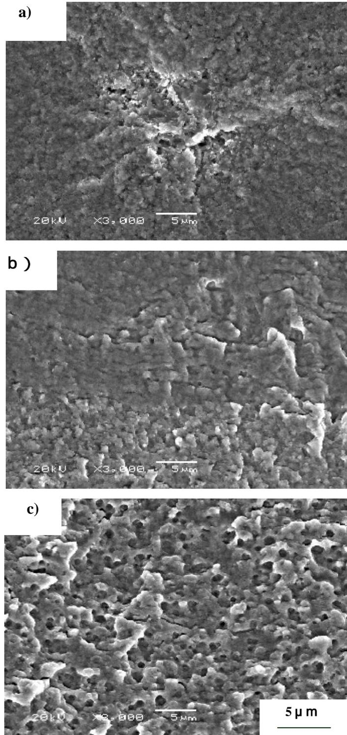
Fig.6 Fatigue fracture surface of Fe-13Cr-8Ni-2Mo-1Zr steel.
