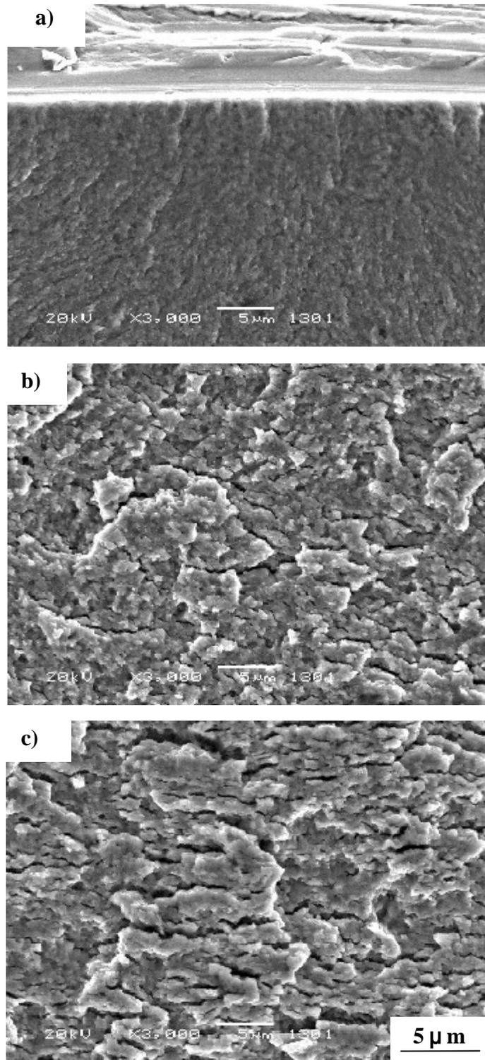
Fig.5 Fatigue fracture surface of Fe-2.25Cr-1Mo-1Zr steel.
