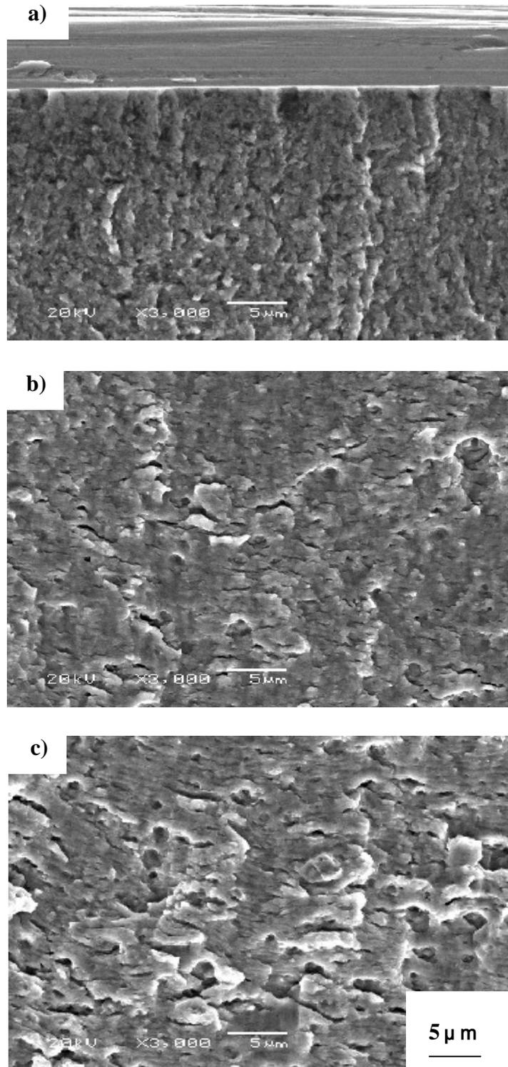
Fig.7 Fatigue fracture surface of Fe-25Cr-1Zr steel
