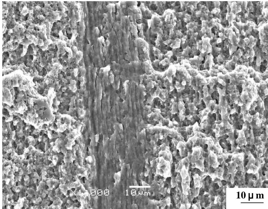
Fig.8 Transgranular fracture surface and striation like pattern observed in crack propagation area of ultra-fine grained Ti-6Al-4V alloy.
