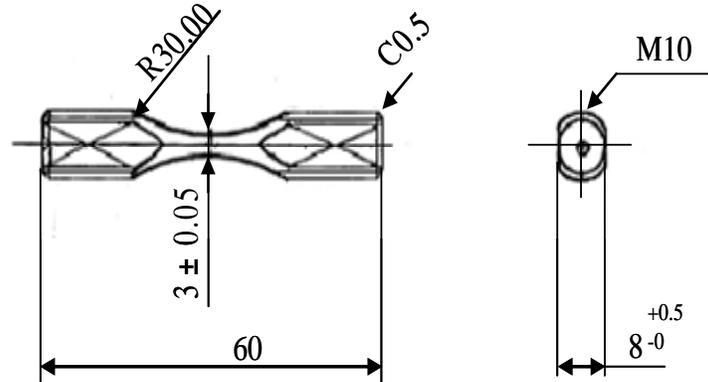
Fig.3 Fatigue test specimen.
