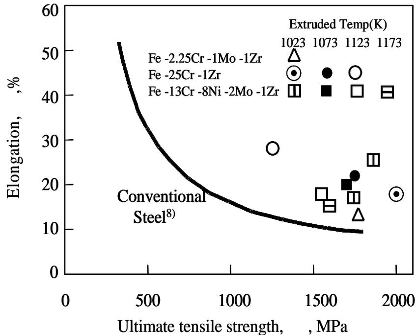
Fig. 2 Relationship between ultimate tensile strength and elongation of ultra-fine grained ferritic stainless steel.
