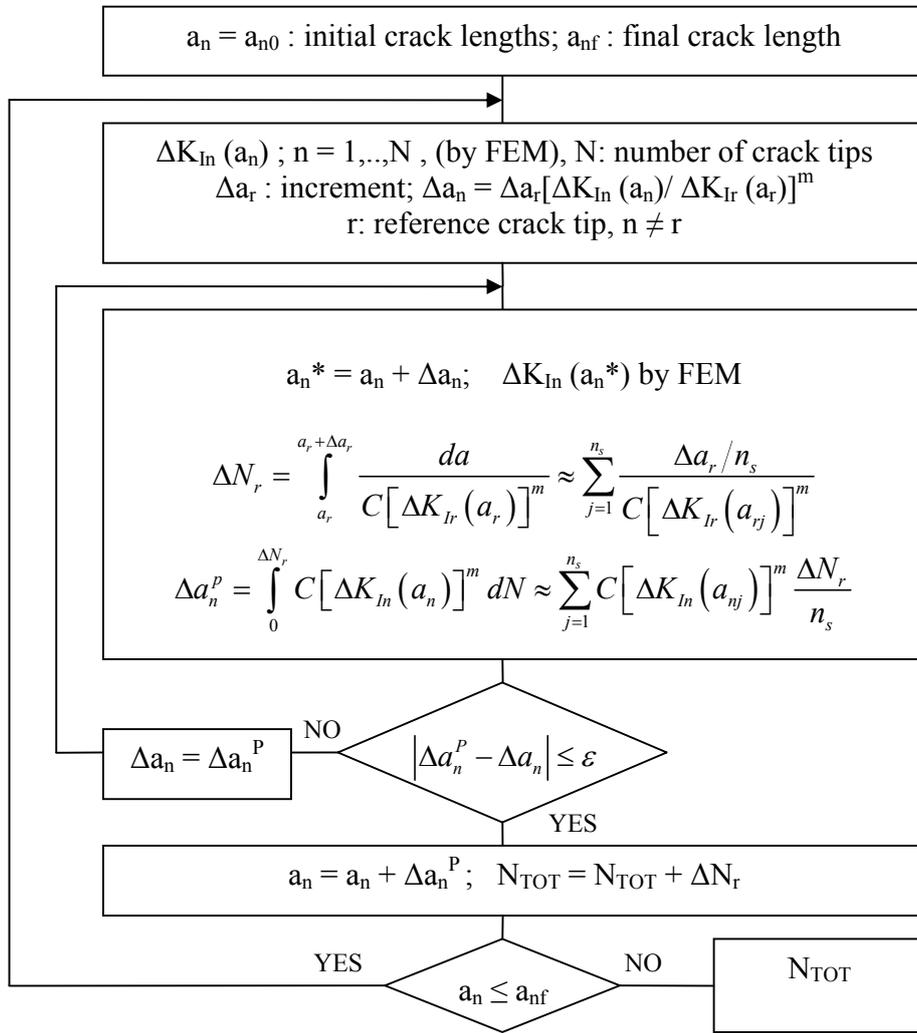
Figure 7. Incremental crack growth simulation procedure for multiple propagating crack tips.
