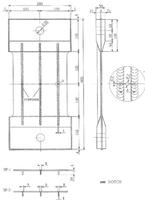
Fig. 2. Stiffened panel specimens SP-1 and SP-3.
