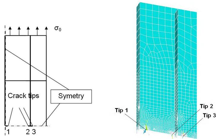
Fig 5. FE boundary conditions and mesh of SP-3 specimen
