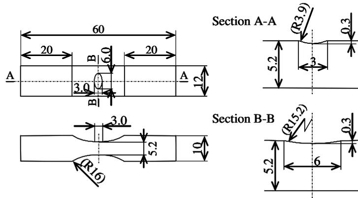
Fig.2 Shape and dimensions of specimen.
