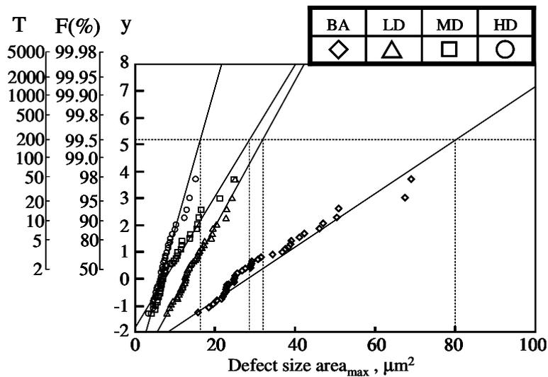
Fig.8 Estimation of defect size by the statistics of extreme value.
