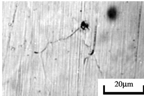
Fig.7 Micro crack from surface defect in Material HD
