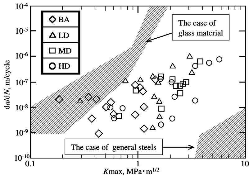
Fig.6 Relationship between stress intensity factor and fatigue crack growth rate.
