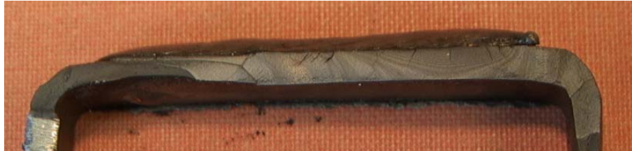
Figure 7 Typical variable amplitude fatigue fracture surface, VA3 spectrum laser peened
