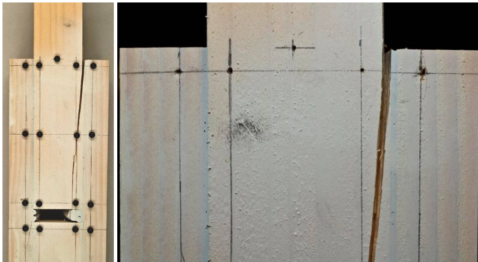
Figure 3: Double-lap specimens after testing: general view (left), close-up at the locus of failure initiation (right)
