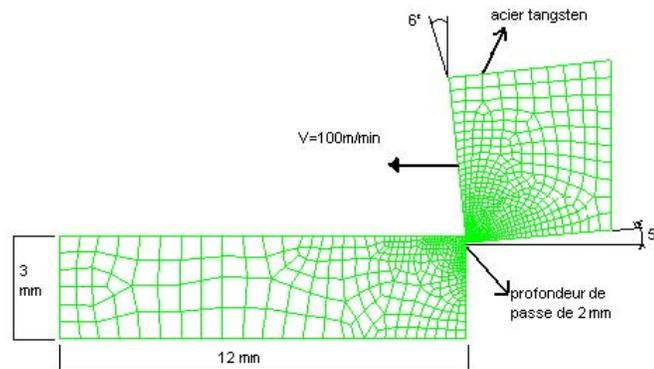
Fig. 1 Orthogonal cutting (initial mesh). The tool is meshed using the same element type and is supposed purely thermoelastic solid define by:  $E=450\,000$  MPa,  $\nu=0.22$ ,  $C_v$
