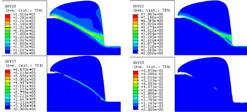
Fig.2: Distribution of some thermomechanical fields at 0.19 mm displacement of the tool.
