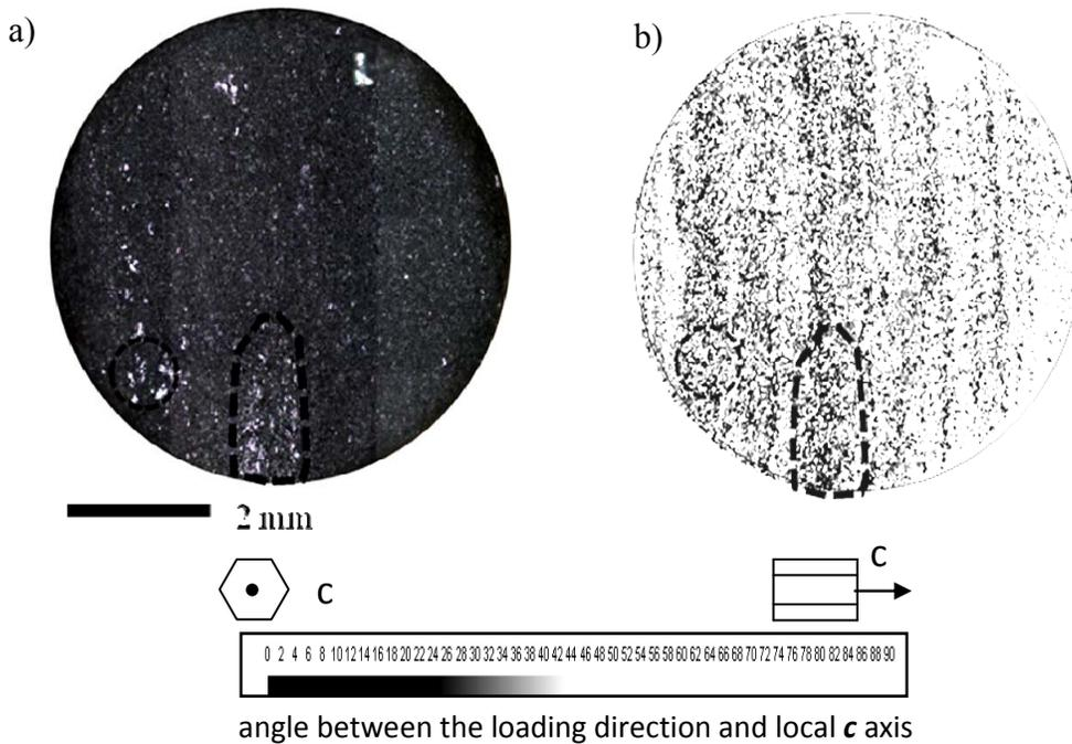
Fig. 1. (a) Optical fractography of a specimen showing a fish eye feature and (b) the EBSD map 100µm below the primary nucleation site showing the presence of macrozones (the grey intensity is related to the angle between the c axis of the crystal and the solicitation direction - SD)
