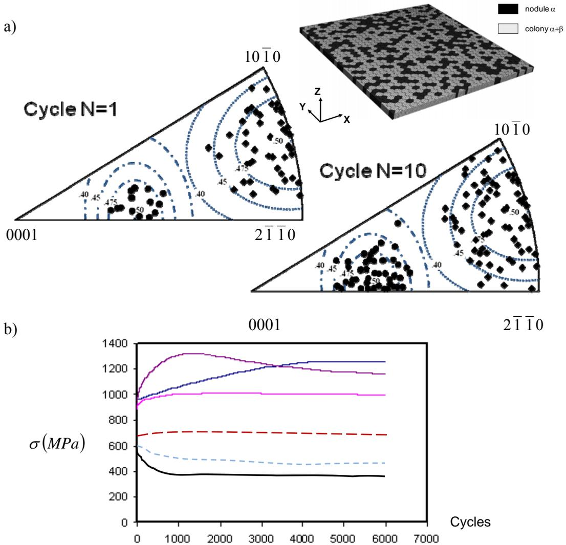
Fig. 5. Micromechanics in fatigue (a) and dwell fatigue (b) investigated by: a) crystal plasticity and inverse pole figures displaying which slip system has been activated after 1 and 10 cycles; and b) cellular automata showing how the local stress may vary according to their orientations, environments and the number of cycles.
