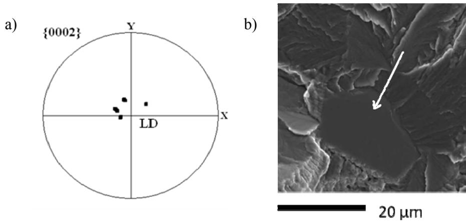
Fig. 3. Nucleation sites; a) pole figure of several nucleation sites; b) an example of a nucleation site (pure cleavage facet) – white arrow.
