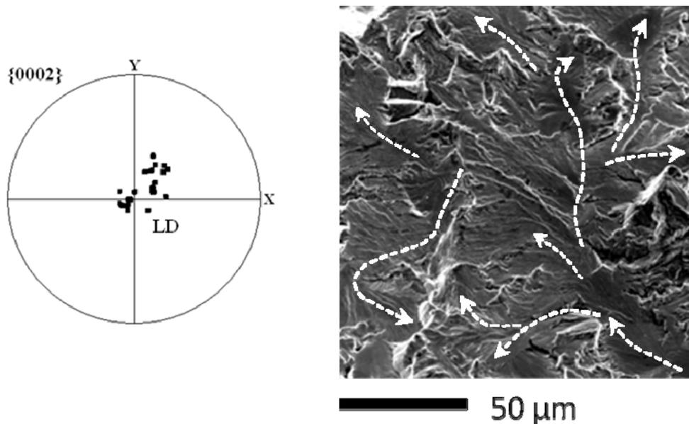
Fig. 4. Propagation path; a) pole figure of quasi cleavage regions along the propagation path; b) example of propagation path (note river marks).
