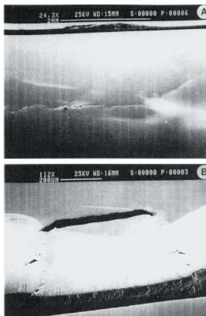
Fig. 1. Two types of HIC: (a) center line cracks, and (b) blister crack.
