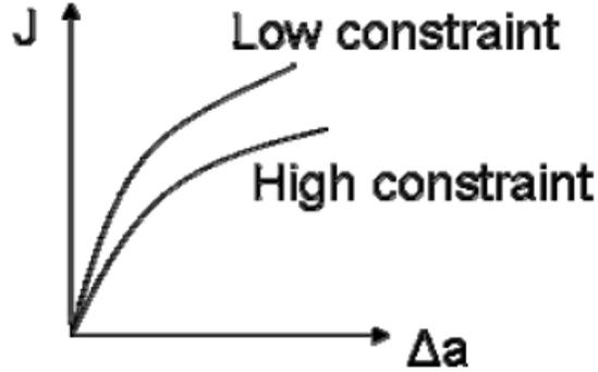
**Fig. 1** Constraint effect on R-curves
