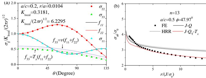
Fig. 2. (a) The elastic stress components of semi-elliptical surface crack front line at  $\phi=45.14^\circ$ , (b) The description of elastic-plastic stress parameters  $\sigma_{\theta\theta}/\sigma_0$  of semi-elliptical surface crack front line.
