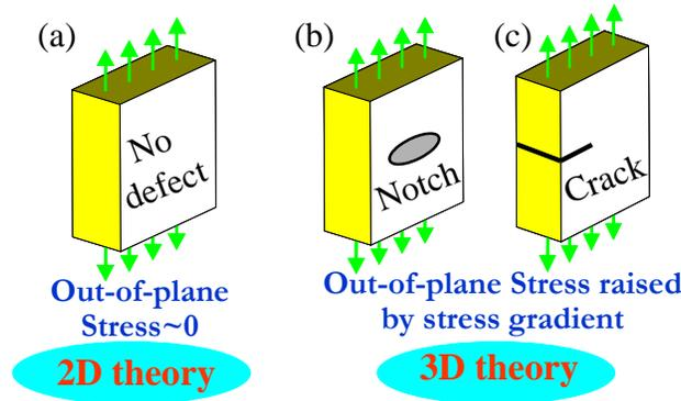
Fig. 1. Finite thickness plates under in-plane loading.
