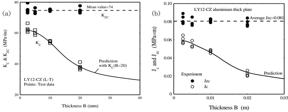
Fig. 3. Variation of two- and three- dimensional fracture toughness parameters  $K_C$ - $K_{ZC}$  (a) and  $J_C$ - $J_{ZC}$  (b) with thicknesses of test specimens.
