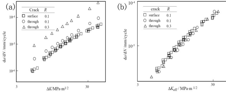
Fig.6  $da/dN \sim \Delta K$  (a) and  $da/dN \sim \Delta K_{eff}$  (b) curves of 20CrMo steel.
