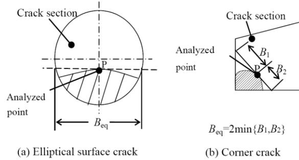
Fig.5. Definition of equivalent thickness  $B_{eq}$  for 3D cracked bodies.
