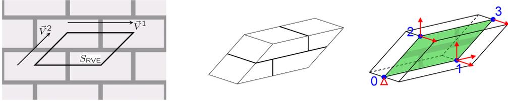
Figure 1: Periodic masonry structure (left) and controlling degrees of freedom (right), see [3].
