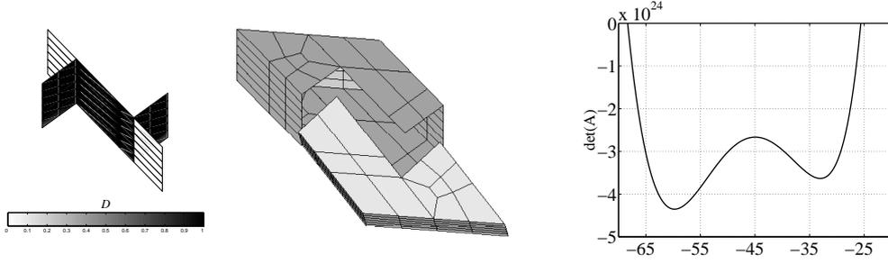
Figure 2: Out-of-plane stair-case bending failure at  $45^\circ$  (brick shape factor of 0.5): joint damage distribution (left), Deformed shape of the unit cell (centre) and related acoustic tensor determinant spectrum (right): non positive values indicate orientation for potential localisation, where the local maximum exactly matches the fine scale-motivated orientation.
