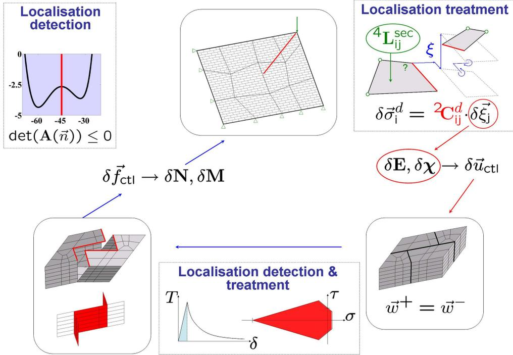
Figure 3: Outline of the complete multi-scale localisation-enhanced scheme
