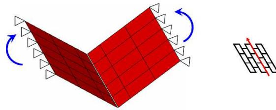
Figure 5: Application: bed joint out-of-plane failure mode (left) and bed joint orientation (right).
