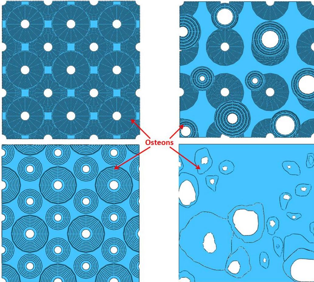
Figure 3. Four different geometry models (extruded to a depth of 0.125 mm) created using the developed code and Abaqus. The code allowed for desired material properties to be assigned to each region. Each model shown measures 0.9 mm across.
