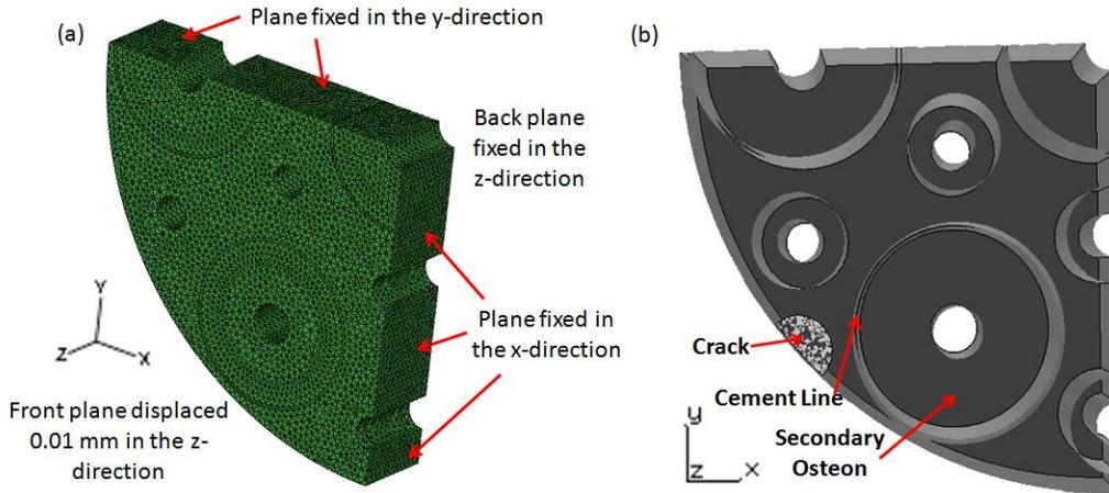
Figure 2. (a) Model with description of boundary conditions. (b) Model showing an inserted crack (image is depicting internal model conditions)
