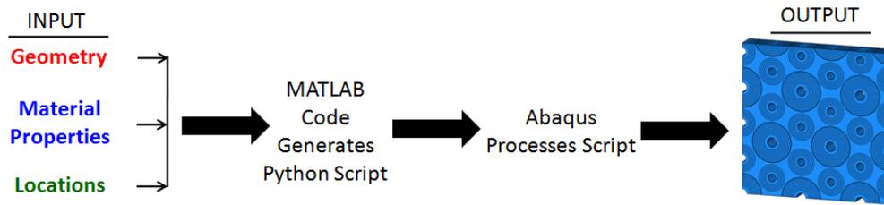
Figure 1. Illustration of model creation procedure
