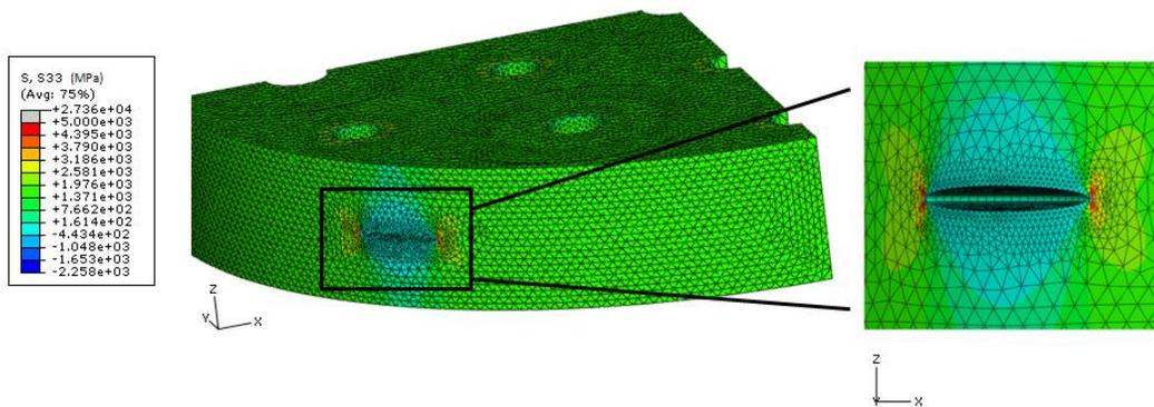
Figure 4. Results from a stress analysis performed on the example microstructural model with the propagated crack (height of quarter cylinder is 0.125 mm)
