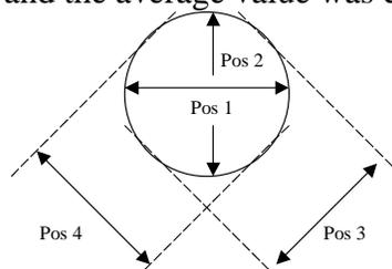
Figure 1 – Position of housing size analysis
