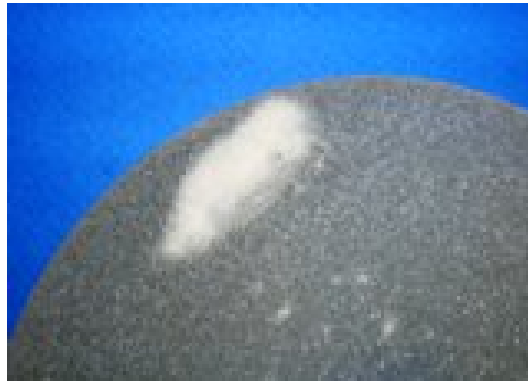
Figure 5 – Representative macroscopic image of a spot inside the silicon shell of a breast implant explanted from a patient subjected to radiation therapy
