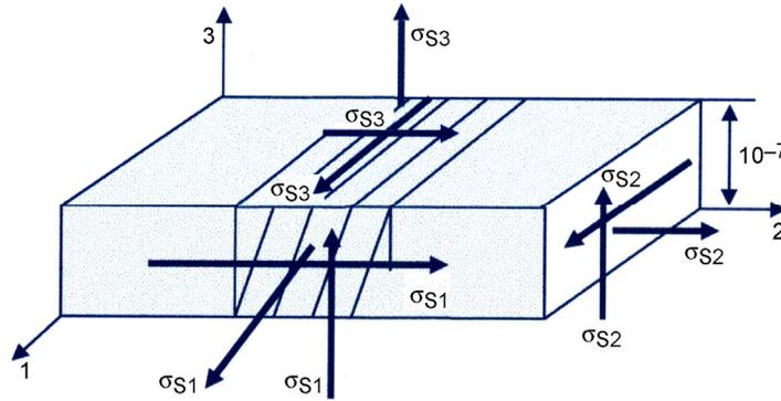
Fig. 4. Nanostresses on a nanosubply (units are in in.).
