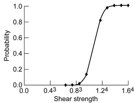
Fig. 12. Probabilistically plotted intralaminar uniaxial shear strength.
