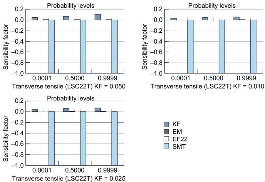
Fig. 13. Probabilistic sensitivities for nanouniaxial transverse tensile strength for three different probabilities.
