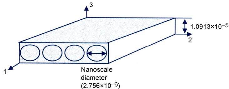
Fig. 2. Nanoscale isolation of a typical part (units are in in.).
