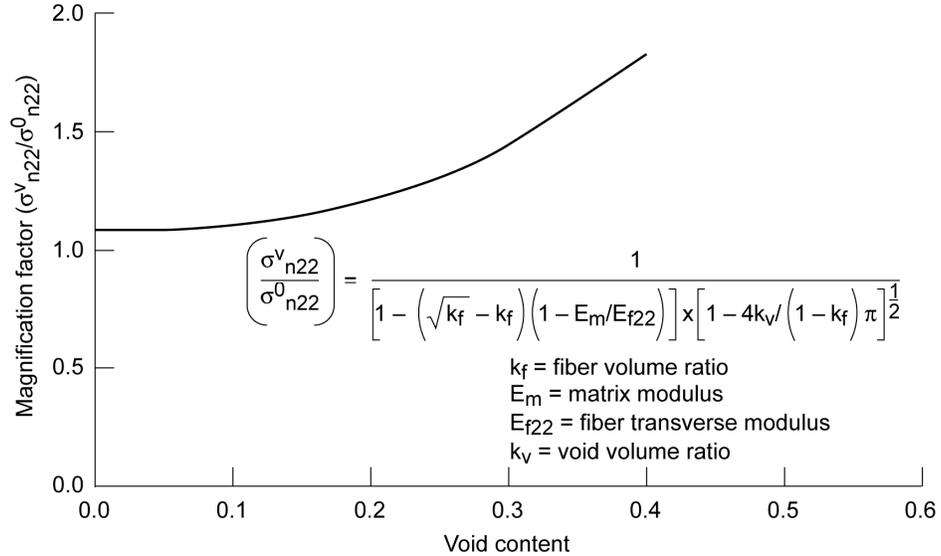
Fig. 6. Nanocomposite magnification factor.
