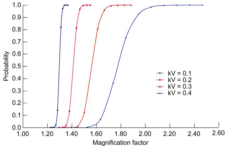
Fig. 7. Probabilistic magnification factor of voids in the interphase.
