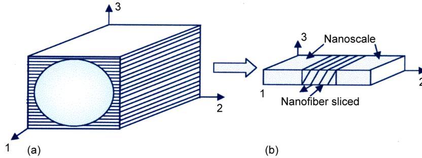
Fig. 3. Nanofiber substructuring. (a) Several slices through the thickness. (b) Nanofiber sliced.
