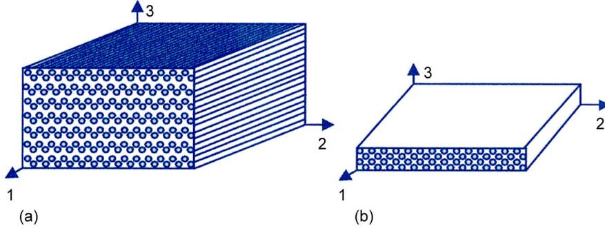
Fig. 1. Unidirectional nanocomposite typical section. (a) Nanocomposite. (b) Nanoply.
