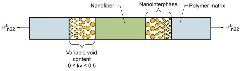
Fig. 5. Vertical section a composite nanocell through nanofiber center.
