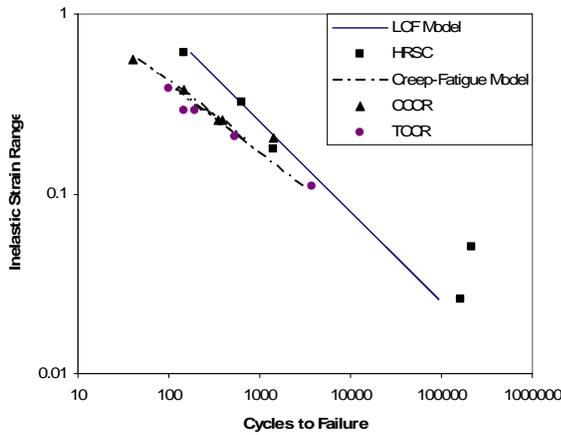
Figure 4. Comparisons of Eq. (9) with experimental data for Rene 80 at 871°C.
