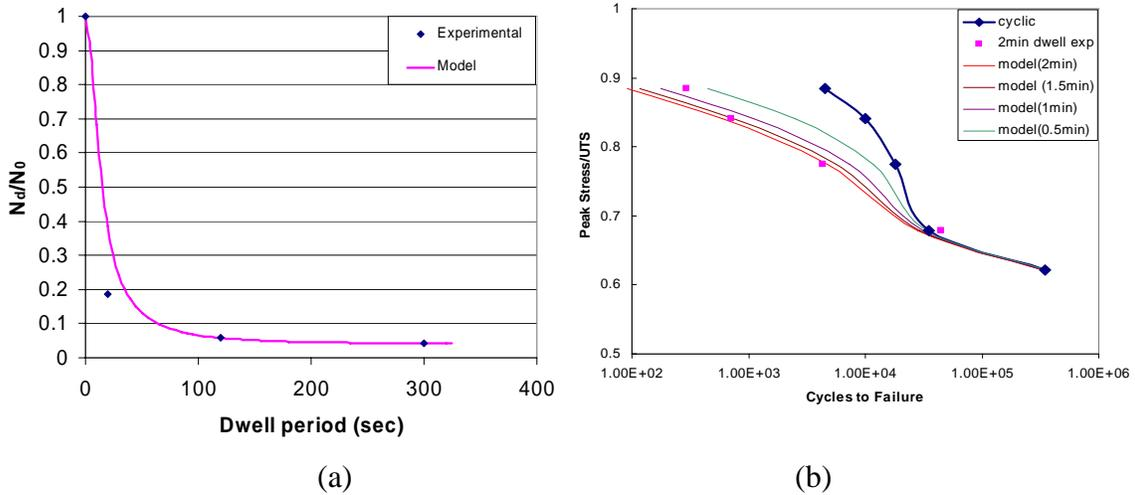
Figure 3. Comparison of Eq. (8) with the experimental data on IMI 834 [14]: a) Normalized dwell fatigue life as a function of dwell time, b) S-N curves with different dwell times.
