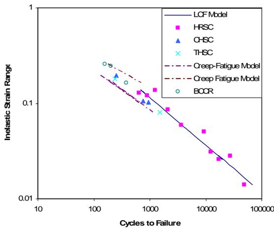
Figure 5. Comparisons of Eq. (9) with experimental data for IN 100 (coated) at 1000°C.
