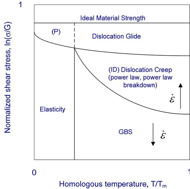
Figure 1 : Schematic deformation mechanism map.
