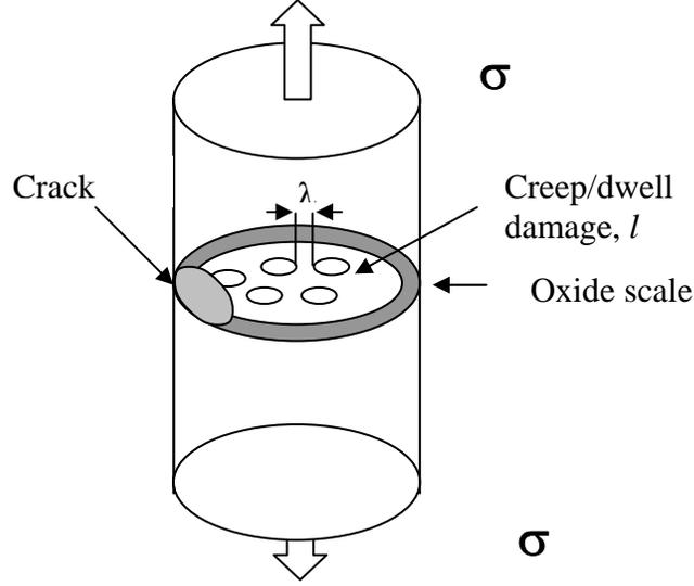
Figure 2. A schematic of damage development in a specimen cross-section.
