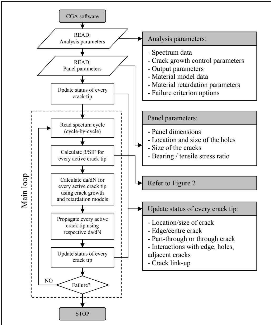
Figure 3. MSD crack growth analysis procedure.
