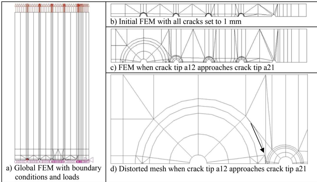
Figure 7. StressCheck finite element model.
