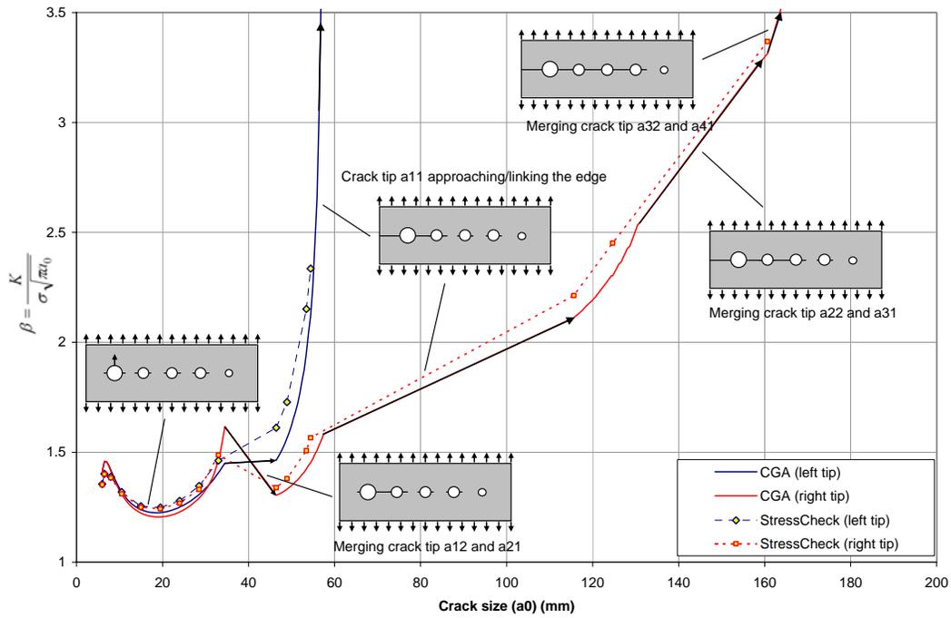
Figure 5. Comparison between the lead crack ( $a_{11} / a_{12}$ )  $\beta$ -solutions obtained using NRC's CGA software and StressCheck finite element analyses.
