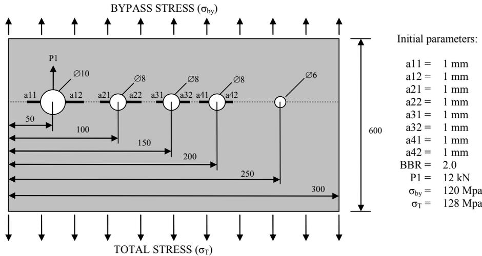
Figure 4. Parametric MSD panel case study. Dimensions are in millimetres (mm).
