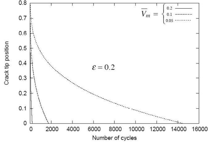
Figure 5. Influence of the amplitude of loading on the debonding evolution
