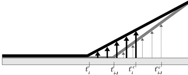
Figure 3. Positions of the crack tip and of the process zone tip at the end of the loading phase of the cycles  $i-1$  and  $i$ .
