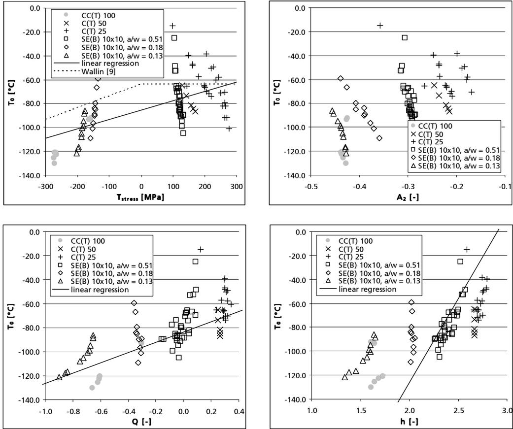
Figure 3: Constraint effect on master curve reference temperature  $T_0$ .
