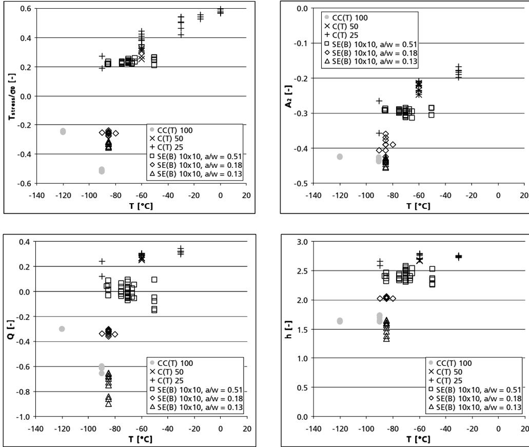
Figure 2: Secondary fracture parameter in dependence on temperature.
