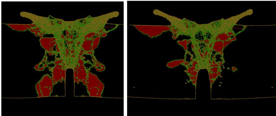
Figure 4 Local crystalline orders at 15.0ps (left) and 20.8ps (right) after impact.
