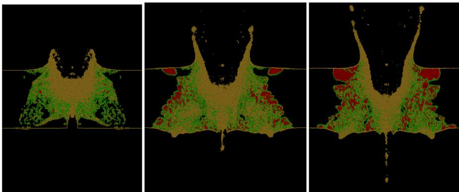
Figure 4 Local crystalline orders at 2.5ps (left), 5.0ps (center) and 7.5ps (right) after impact.
