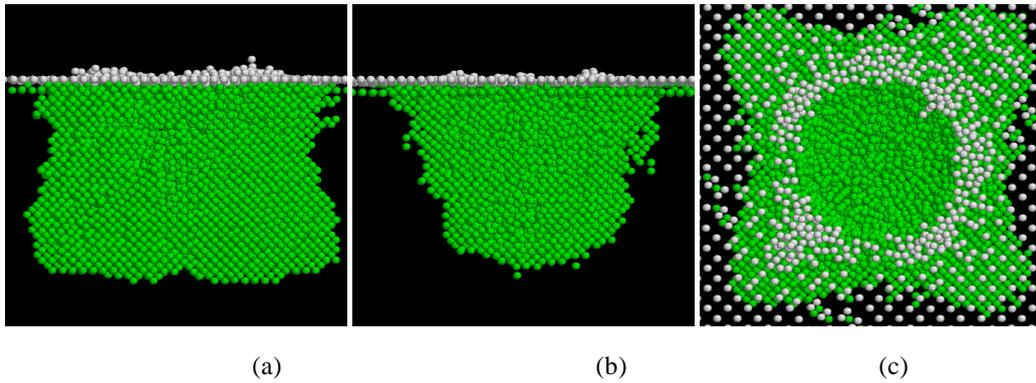
Figure 3 (a-b)Frontal views of local crystalline orders at 1.3ps and 2.5ps after a Si cluster of 260 atoms impacting with a Si substrate. (c)The corresponding top view of graph (a).
