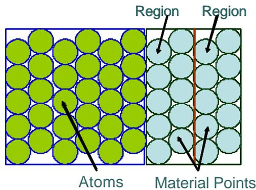
Figure 1 A schematic view of MPM/MD handshaking method. Material points in the handshaking region serve to provide an atmosphere for the atoms within the potential cutoff from the interface.
