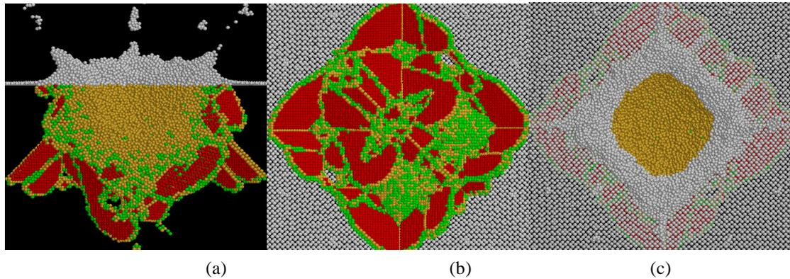
Figure 2 (a)Frontal views of local crystalline orders for 4.2ps after impact for the cluster with 1052 atoms .(b) and (c)The corresponding bottom and top view of graph (a).
