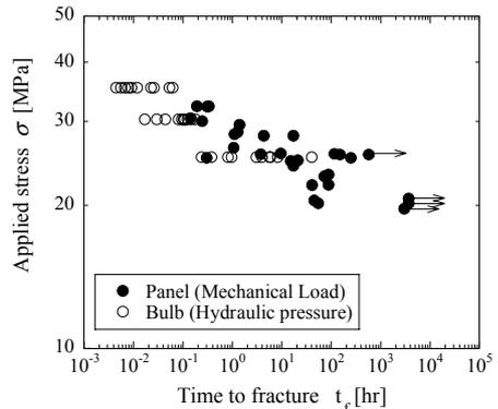
Figure 4: Delayed fracture strength of bulbs and panels
