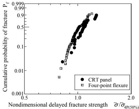
Figure 6: Weibull distribution of non-dimensional delayed fracture strength
