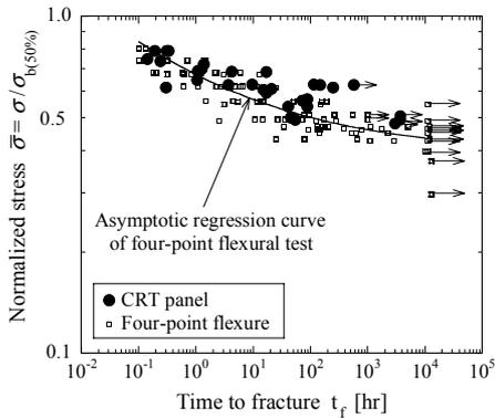
Figure 5: Comparison of delayed fracture properties between glass specimen and panel
