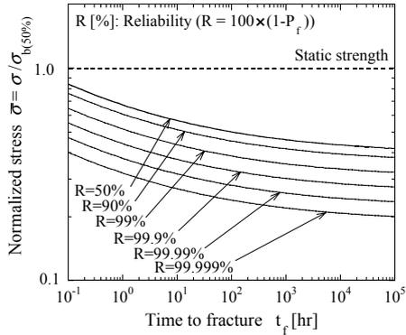
Figure 7: Relationship between reliability and allowable stress normalized by static strength
