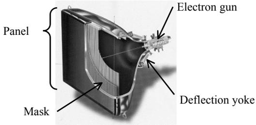
Figure 1: Appearance of CRT bulb
