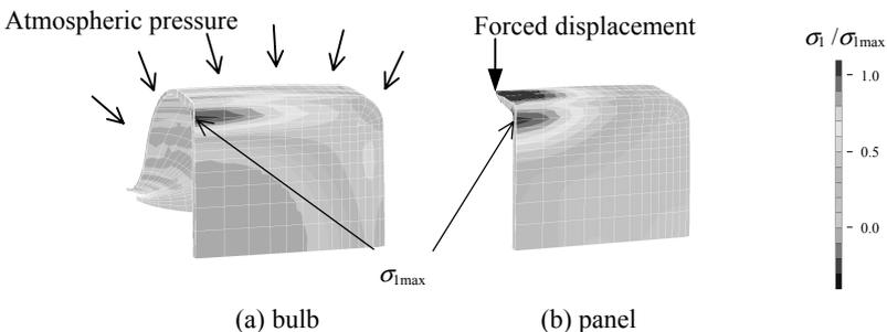
Figure 2: Distribution of maximum principal stress,  $\sigma_1$  (1/4 symmetric model)
