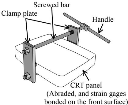
Figure 3: Schematic illustration of clamp jig for CRT panel
