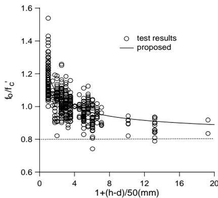
Figure: 1 Relationship between relative concrete strength ( $f_o/f_c'$ ) and  $1+(h-d)/50$ .
