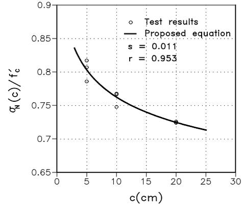
Figure 5: Normalized nominal strength with compressive strength versus depth.
