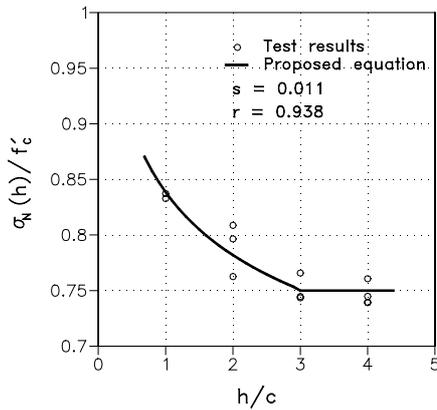
Figure 4: Normalized nominal strength with compressive strength versus ratio of length to depth.
