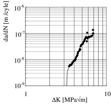
Figure 2:  $da/dN$  versus  $\Delta K$  for the Sc modified alloy in the threshold region.
