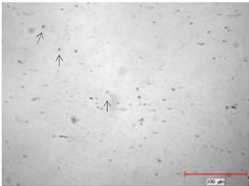
Figure 5: The unetched optical micrograph of the Sc modified alloy showing the  $\text{Al}_3\text{Sc}_x\text{Zr}_{1-x}$  particles  $\uparrow$ .
