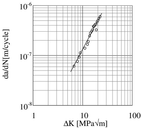
Figure 3:  $da/dN$  versus  $\Delta K$  for the 7010 alloy in the Paris region.
