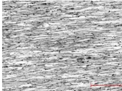
Figure 6: The optical micrograph of the Sc modified alloy showing the elongated unrecrystallized grains.
