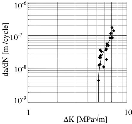
Figure 1:  $da/dN$  versus  $\Delta K$  for the 7010 alloy in the threshold region.
