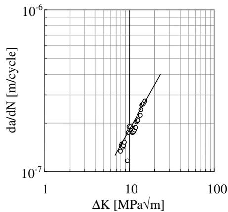
Figure 4:  $da/dN$  versus  $\Delta K$  for the Sc modified alloy in the Paris region.
