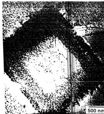
Figure 8: The TEM photograph of the Sc modified alloy showing the cuboidal particle [3].
