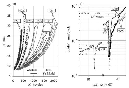
Figure 5: Comparisons between the experimental results and predictions from the SY model according to the present authors: (a) CA tests; (b) OL tests
