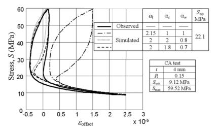
Figure 3: Exemplary comparisons between the observed and simulated P- $\varepsilon_{offset}$  loops for various combinations of the calibration coefficients
