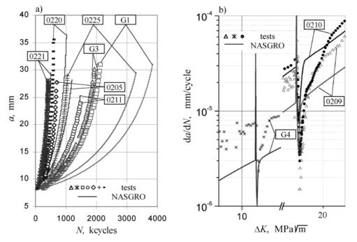
Figure 2: Comparisons between the experimental results and the NASGRO model predictions: (a) CA tests; (b) OL tests
