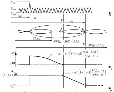
Figure 4: The variations in calibration coefficients within the OL plastic zone
