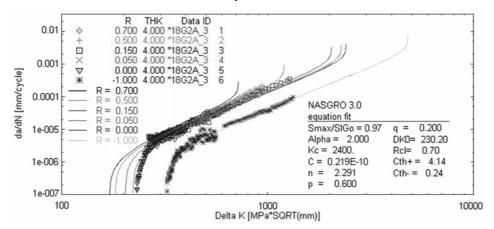
Figure 1: da/dN versus  $\Delta K$  data from the CA tests and the corresponding material parameters used in the NASGRO SY model
