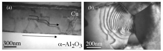
Fig. 3: (a) A threading dislocation gliding on an inclined  $\{111\}_{Cu}$  plane gets constrained between a Cu twin boundary and the film/substrate interface. The advancing dislocation is forced to deposit interfacial dislocation segments at both interfaces (see arrows) [3]. (b) Parallel glide dislocations [4] emitted from a grain boundary in a 150nm thick Cu film during cooling from 500°C to 40°C.
