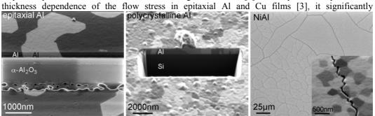
Fig. 1: FIB images of (a) a 350nm thick epitaxial (bicrystal) Al film grown on a (0001)-oriented  $\alpha$ -Al<sub>2</sub>O<sub>3</sub> single crystal [8], (b) a 1000nm thick polycrystalline Al film grown on an oxidised (001) Si substrate [3], and (c) a 1500nm thick Al rich NiAl film (52.2at% Al) on a nitrided (001) Si substrate. Note that cracks are present in the Al rich NiAl film, which run mainly along NiAl grain boundaries (see enlarged inset in (c)) [6].
