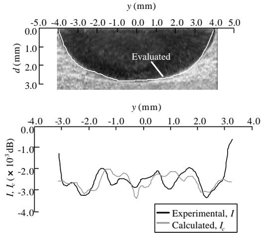
Figure 5: Evaluated distribution of crack depth
