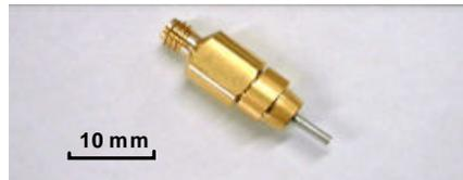
Figure 2: Photograph of the open-ended coaxial line sensor
