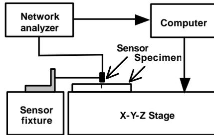
Figure 1: Configuration of the microwave inspection system
