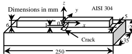
Figure 3: Descriptive geometry of the specimen used to introduce a 3-D crack
