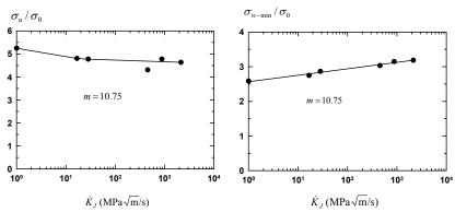
Figure 1: Calibrated variations of  $\sigma_u$  and  $\sigma_{w-min}$  with loading rate.
