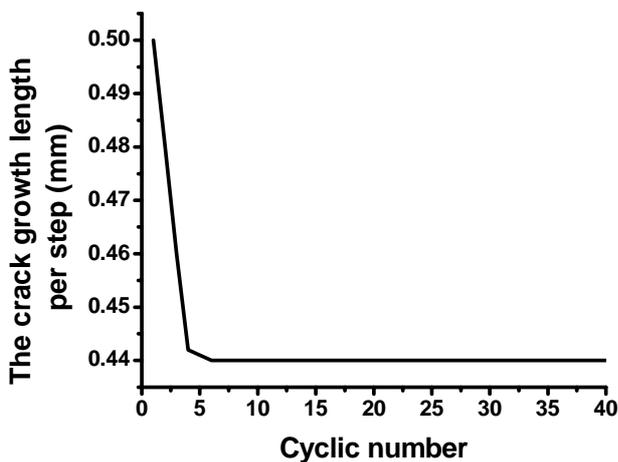
Fig.6 Crack growth per reversal vs. reversal number
