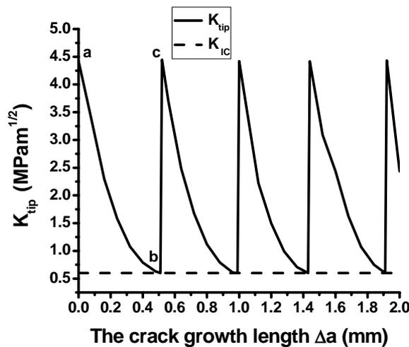
Fig.5  $K_{tip}(\Delta a)$  at the crack tip vs. the crack growth  $\Delta a$
