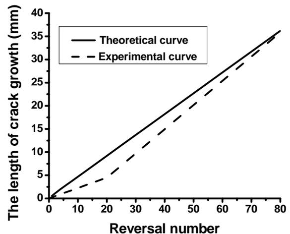
Fig.7 The crack growth vs the reversal number
