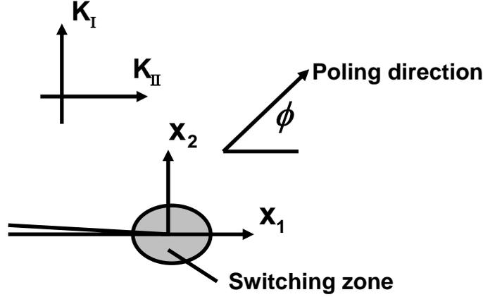
Fig.1 Switching zone near the tip of a crack
