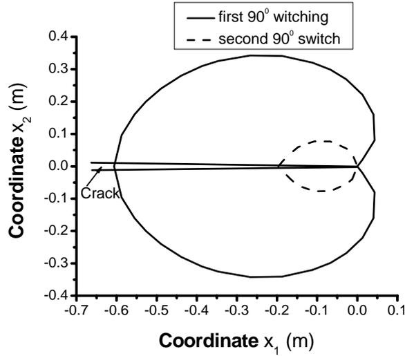
Fig.3 Domain Switchings zones induced by an positive electric field
