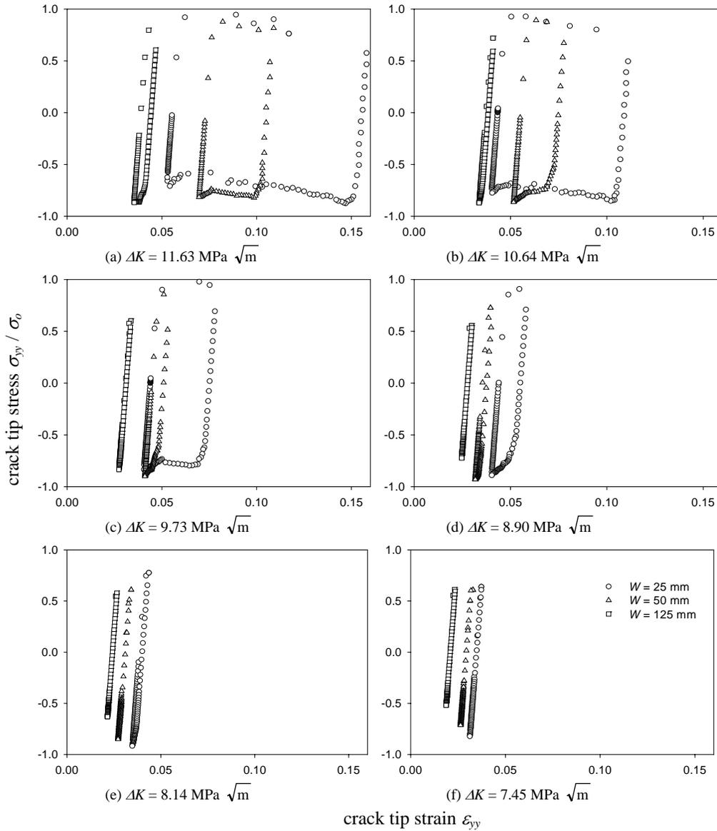
Figure 1: Crack tip hysteresis loops.
