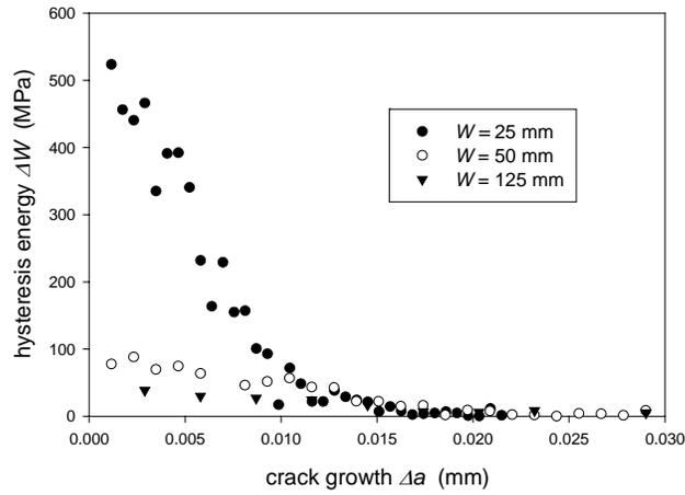
Figure 2: Variation of crack tip plastic strain hysteresis energy.
