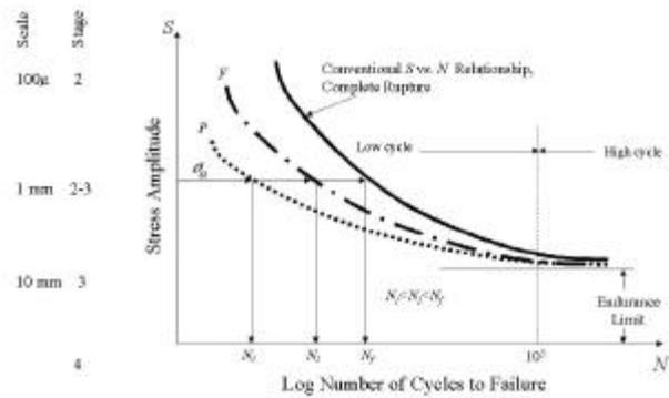
Fig. 2 Conventional representation of fatigue process
