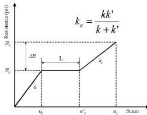
Fig. 4 Response of a single element of model
