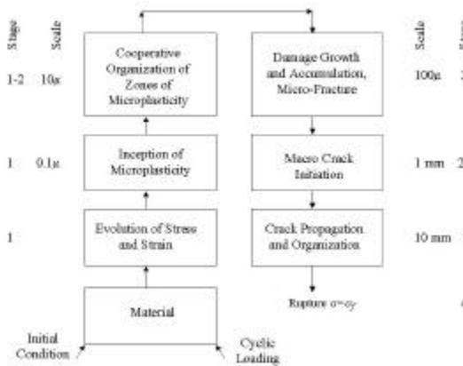
Fig. 1 Stages in progression leading to fatigue fracture or rupture
