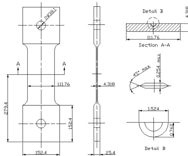
Figure 1: Part-through crack specimen configuration.
