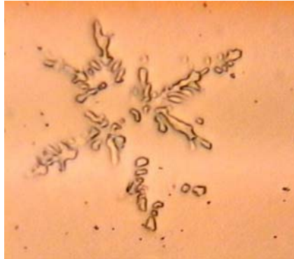
Fig. 1 – Typical dendritic structure in sample A (width of field 30 \mu\text{m} ).
