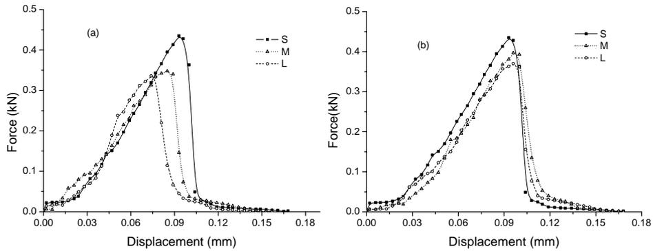
Fig. 2 Load-displacement diagram vs. specimen size before ASR
