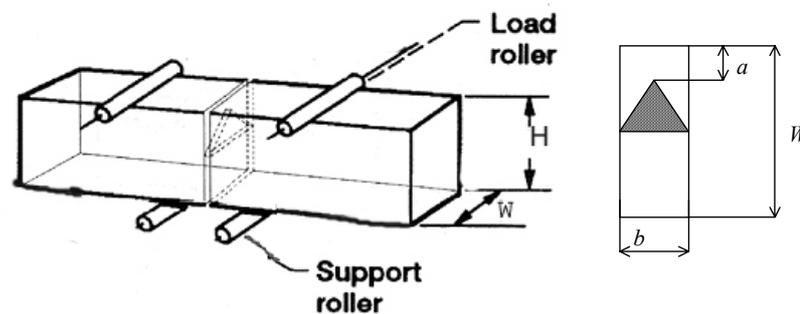
Figure 1. Chevron-notched beam in four-point bend test
