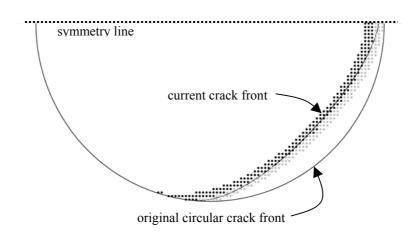
Figure 4: Predicted crack front shapes.
