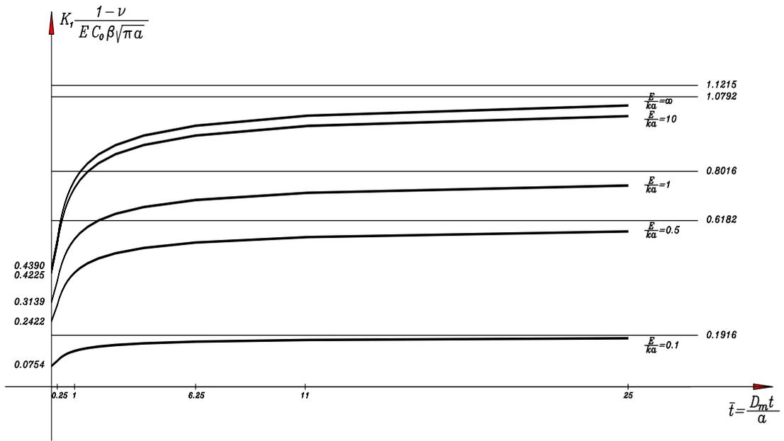
Figure 3: SIF for the reinforced crack during the time for the different values of  $E/ka$
