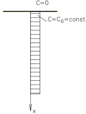
Figure 1: Infinite half-space with the initial moisture distribution
