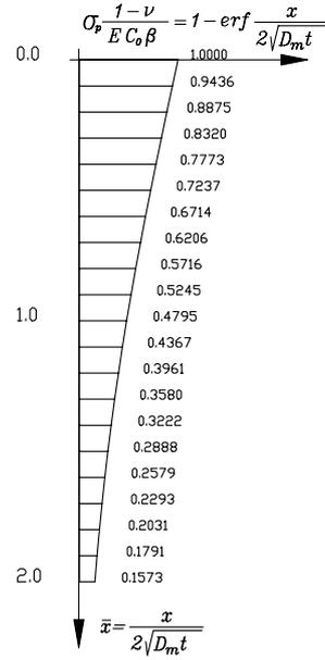
Figure 2: The stress distribution due to moisture change
