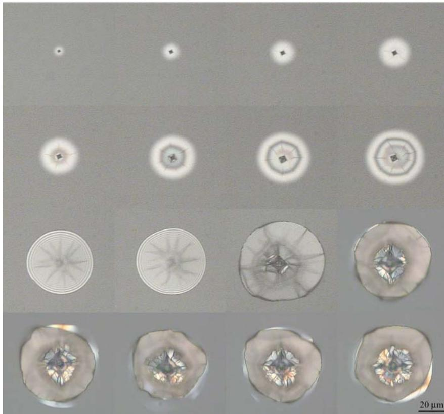
Figure 1: Optical photos to demonstrate the development of indentation-induced delamination in the 1.535  $\mu\text{m}$ -thick ZnO/Si system after indented under 0.05, 0.10, 0.15, 0.20, 0.25, 0.30, 0.35, 0.40, 0.45, 0.50, 0.75, 1.00, 1.25, 1.50, 1.75 and 2.00 N, respectively.
