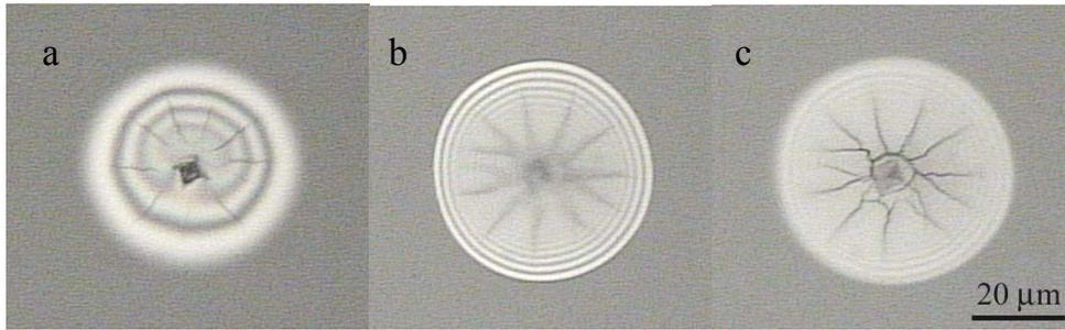
Figure 2: Optical photos to show the development of buckling of the 1.535  $\mu\text{m}$ -thick-ZnO/Si system after indented under the critical load of 420 mN. (a) The state at about two minutes before buckling. (b) Final state after buckling. Focus on the perimeter of the debonded film. (c) Final state after buckling. Focus on the internal circle.
