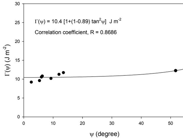
Figure 3: Fitting experimental data of the interfacial fracture toughness with the empirical formula,  $\Gamma(\psi) = \Gamma_i^c [1 + (1 - \lambda) \tan^2 \psi]$ , to extract the value of  $\Gamma_i^c$ .
