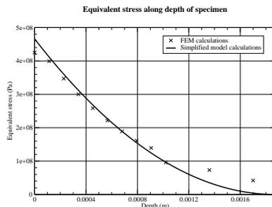
Figure 4: Comparison between FEM and simplified model calculations
