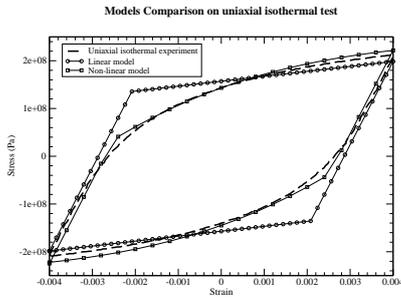
Figure 5: Models comparison on uniaxial isothermal test
