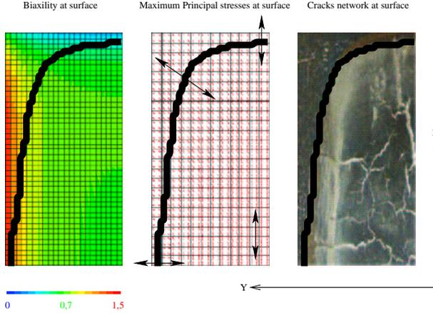
Figure 7: Results from elastic calculations
