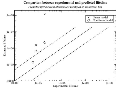
Figure 8: Fatigue lifetime estimation
