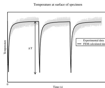
Figure 3: Thermal transient
