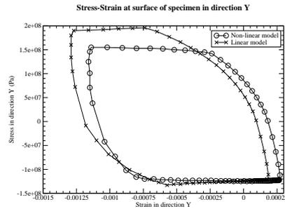
Figure 6: Models comparison on SPLASH stabilized cycle
