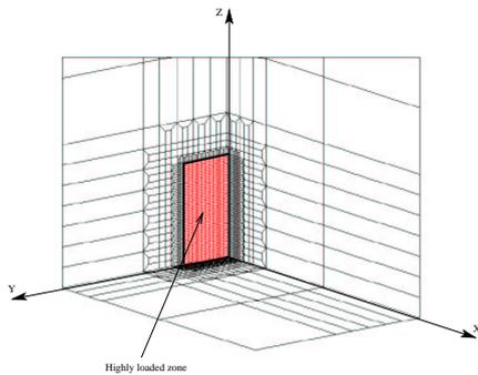
Figure 2: SPLASH specimen mesh
