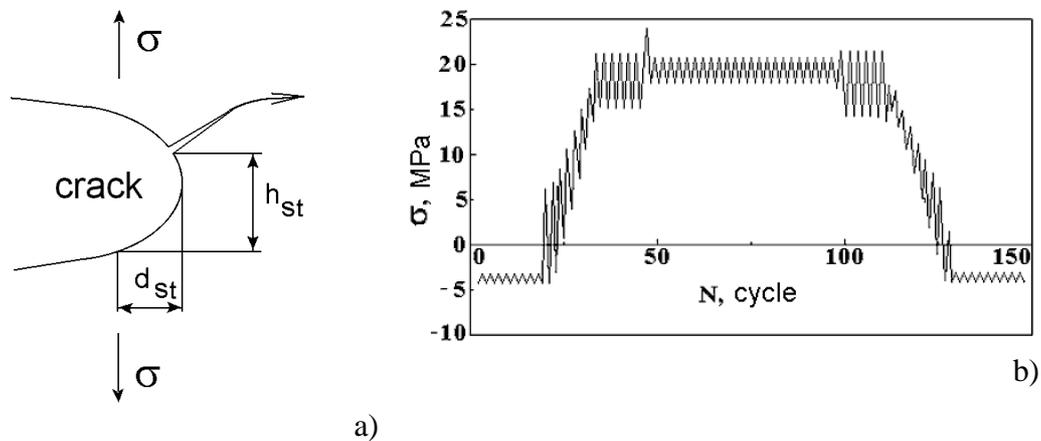
Figure 2: Parameters (a) for schematized stretched zone, and (b) schematized block of cyclic loads by flight, which was discovered in the wing of the aircraft Yak-42.
