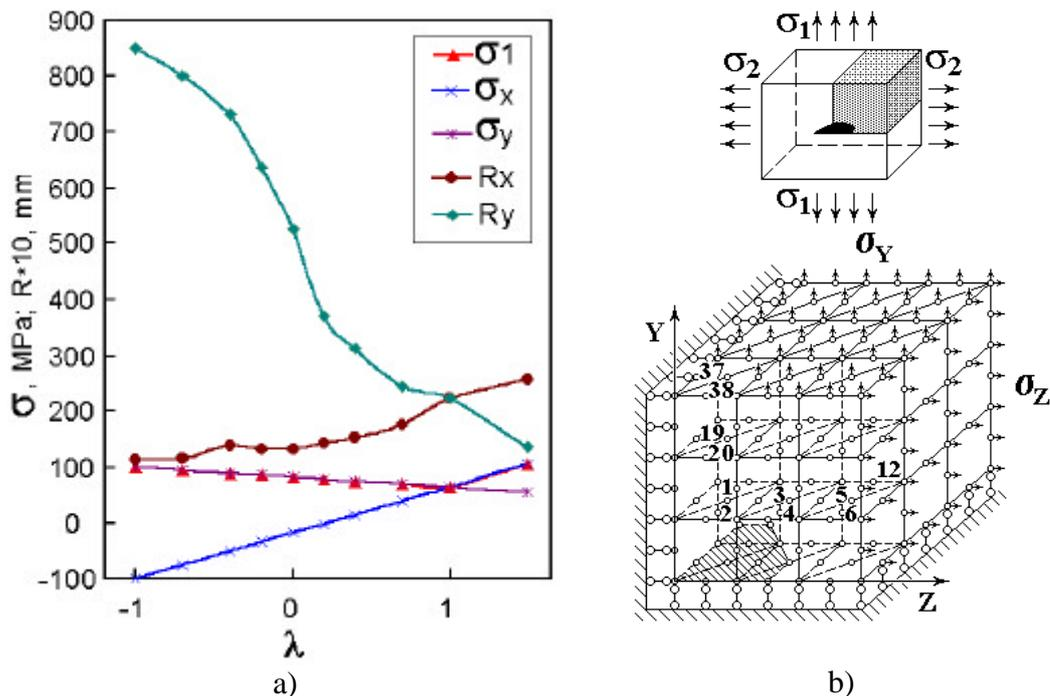
Figure 1: Results of FEM analysis (a) for stress-state estimation and radius  $R_x$ ,  $R_y$  for uniformly stress state of the cruciform specimen in 5 mm of the thickness, and (b) periodic cells used in the cruciform specimen of the 10 mm in the thickness for the semi-elliptical crack.
